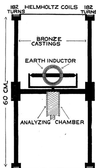
Fig. 2. Arrangement of Helmholtz coils.
