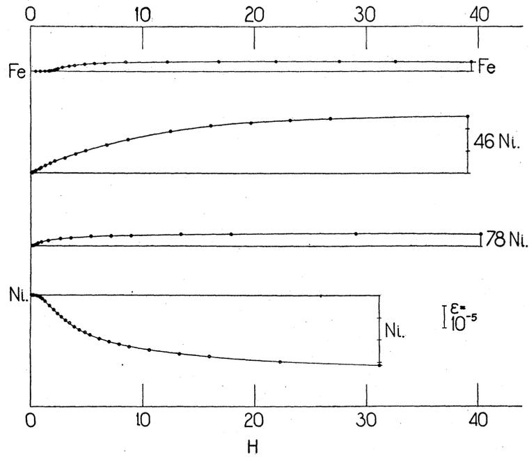
Fig. 4. The strain  $\epsilon$  as a function of magnetic field strength.
