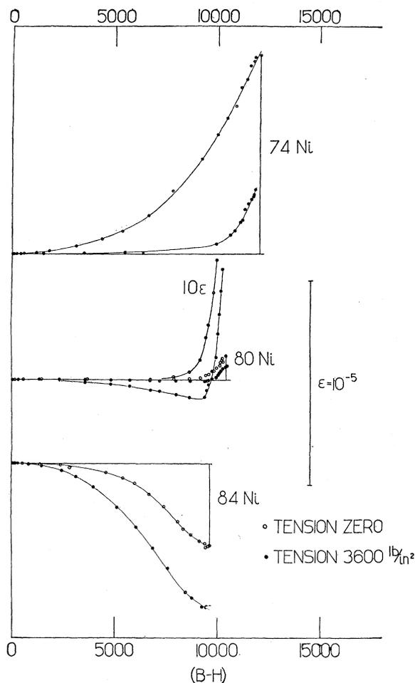
Fig. 6. Showing results for magnetostriction in stretched permalloys.
