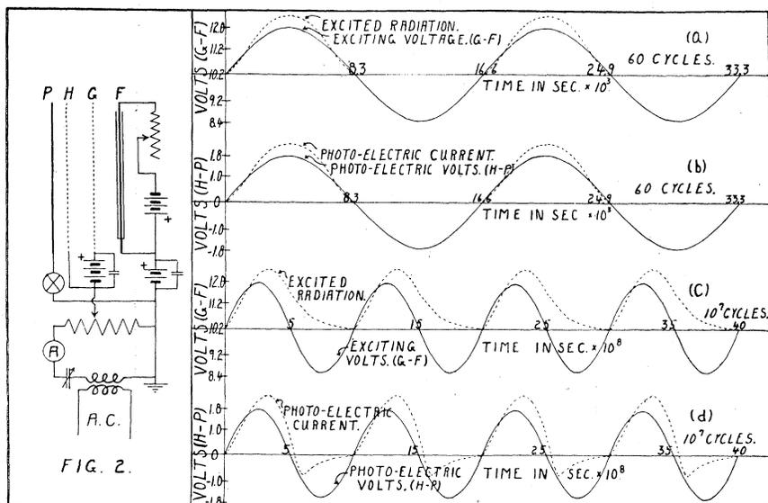
Fig. 2. Electrical connections for persistence measurements. Curves (a), (b), (c), and (d) show the processes involved in measurements.
