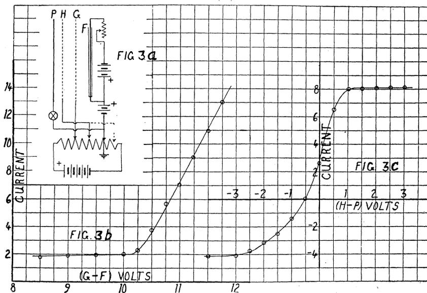
Fig. 3a. Electrical connections for d.c. characteristics.
