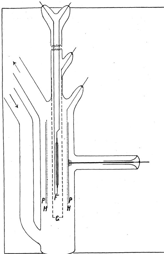
Fig. 1. Schematic diagram of experimental tube 2. Drawn to scale.
