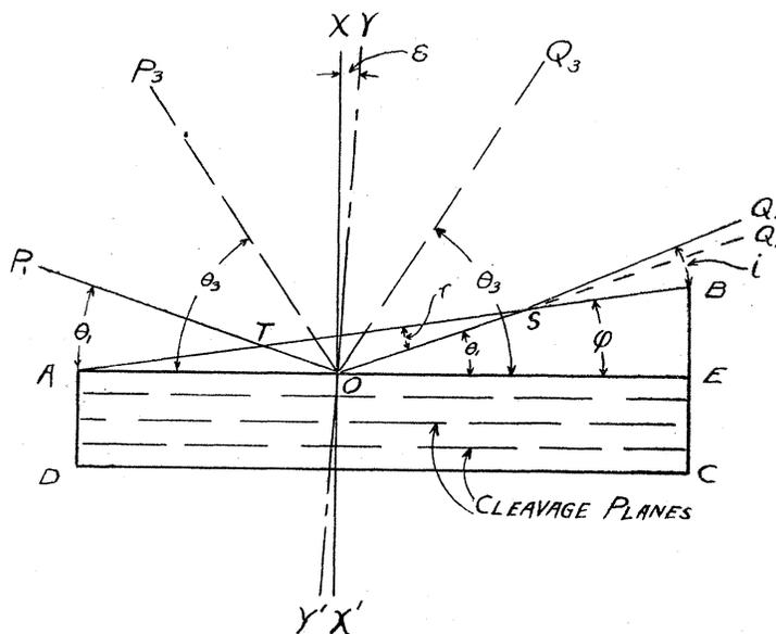
Fig. 1. Paths of rays in wedge method.
