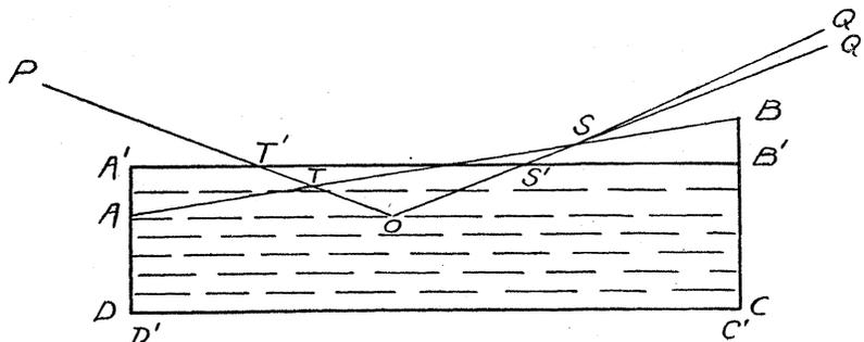
Fig. 2. Paths of rays in differential wedge method.
