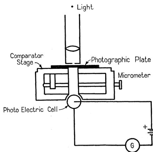
Fig. 2. Photo-electric spectro-photometer.
