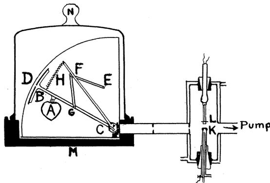
Fig. 1. Vacuum x-ray spectrograph.
