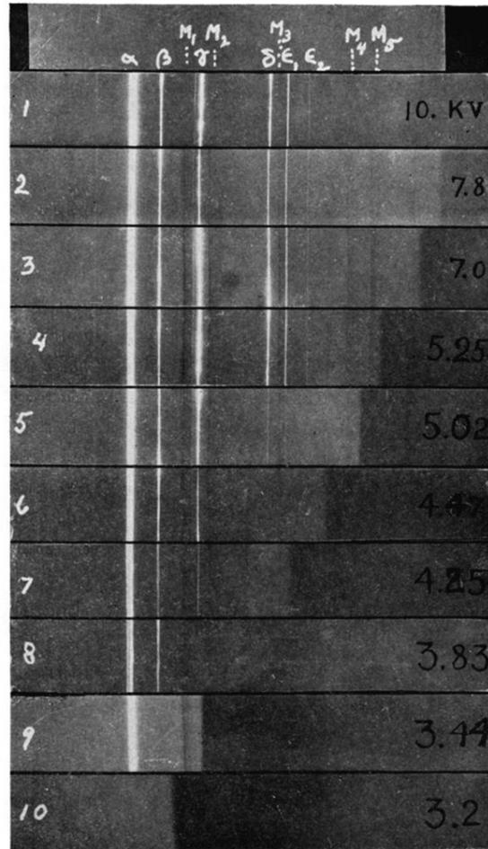
Fig. 2. Spectrograms taken with various potentials decreasing from 10kv to 3.2kv.
