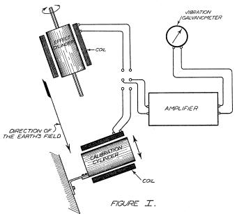
The general arrangement of the apparatus is shown schematically in Fig. I. The potential produced in the secondary by the rotary oscillations of the "effect cylinder" was impressed on a three-stage amplifier, and the amplified current was sent to a vibration galvanometer tuned to the frequency of oscillation.
