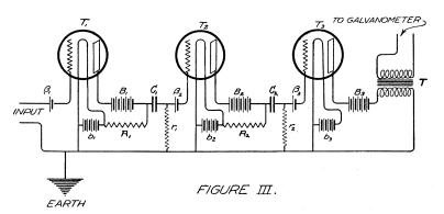
of the impressed electromotive force was low, resistance coupling instead of transformer coupling was used between the stages.
