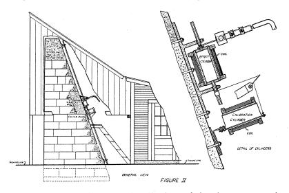
feet, two feet being below ground. The base of the pier was seven feet from face to back, five feet wide at the face and three feet wide at the back. The cap of the pier was not quite two feet from face to back and three feet wide. It will thus be seen that the structure was quite massive and solid.
