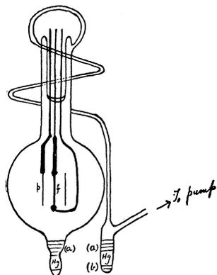
the parts which contained no liquid mercury always at a temperature about 100 degrees higher than that of the reservoirs, the reason being to prevent any condensation from taking place in these regions.
