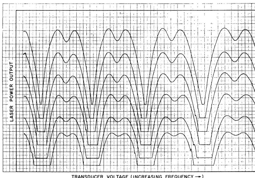
500 V to this transducer allowed tuning through 3 adjacent modes. The cavity length versus transducer voltage had a 3% nonlinearity. However, this was wholly reproducible and was compensated for in the data handling.
