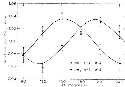
FIG. 1. Perturbed angular correlation of the 40–141-keV  $\gamma$ - $\gamma$  cascade in  $^{99}Tc$ . The source was in the form of a dilute alloy of Mo with Fe. The two curves correspond to the two directions of the external polarizing field.
