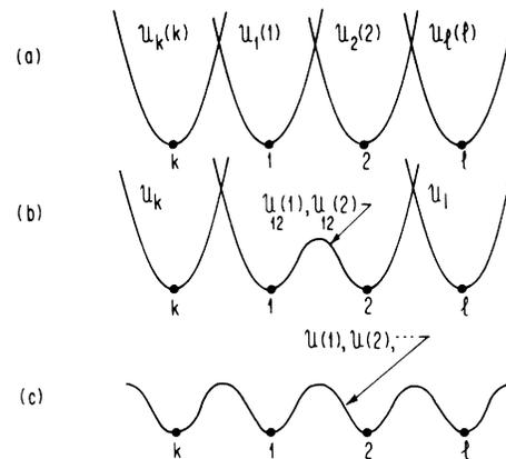
FIG. 1. Single-particle potentials I: (a) Each particle stays in the vicinity of its lattice site — no exchange. (b) Particles 1 and 2 can exchange. They see a common double well due to the other particles in the solid. (c) A periodic single-particle potential is seen by all of the particles in the solid.
