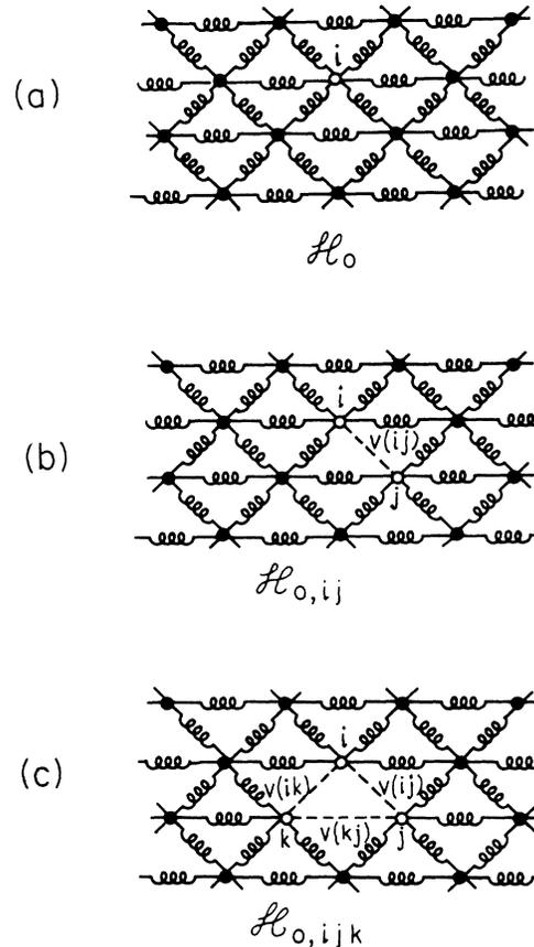
FIG. 3. Springs: (a) In the lowest approximation all of the particles are coupled together by springs. (b) For a pair of particles  $(ij)$  the spring  $w_{ij}(ij)$  is replaced by the Lennard-Jones potential  $v(ij)$ . (c) For a triplet of particles  $(ijk)$  the springs  $w_{ij}(ij)$ ,  $w_{jk}(jk)$ , and  $w_{ki}(ki)$  are replaced by the Lennard-Jones potentials  $v(ij)$ ,  $v(jk)$ , and  $v(ki)$ .
