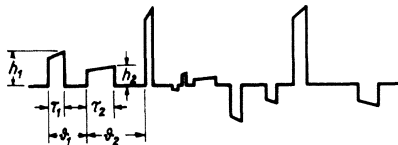
FIG. 2. Pulse sequence with variable parameters \vartheta , \tau , and h .
