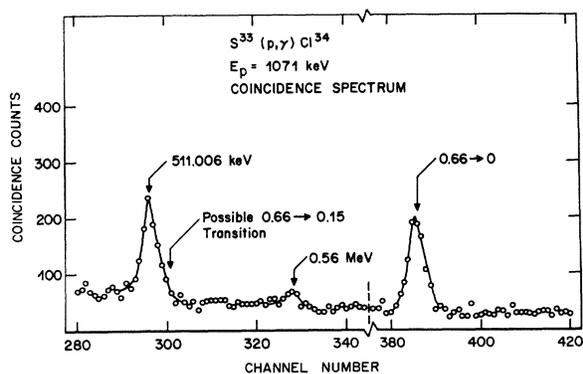
FIG. 3. Selected portions of the Ge(Li)-NaI(Tl) coincidence spectrum at the  $E_p=1071$ -keV resonance. The arrow near channel 300 shows where a peak corresponding to a possible 0.66 $\rightarrow$ 0.15 transition would appear (see text).
