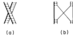
FIG. 5. The thick lines represent protons and, the thin lines, electrons. The ladders represent hydrogen atoms. The dashed lines denote the Coulomb potential responsible for the binding. (a) Exchange of two hydrogen atoms. (b) Exchange of the electrons as a term in the T matrix for the scattering of two hydrogen atoms.
