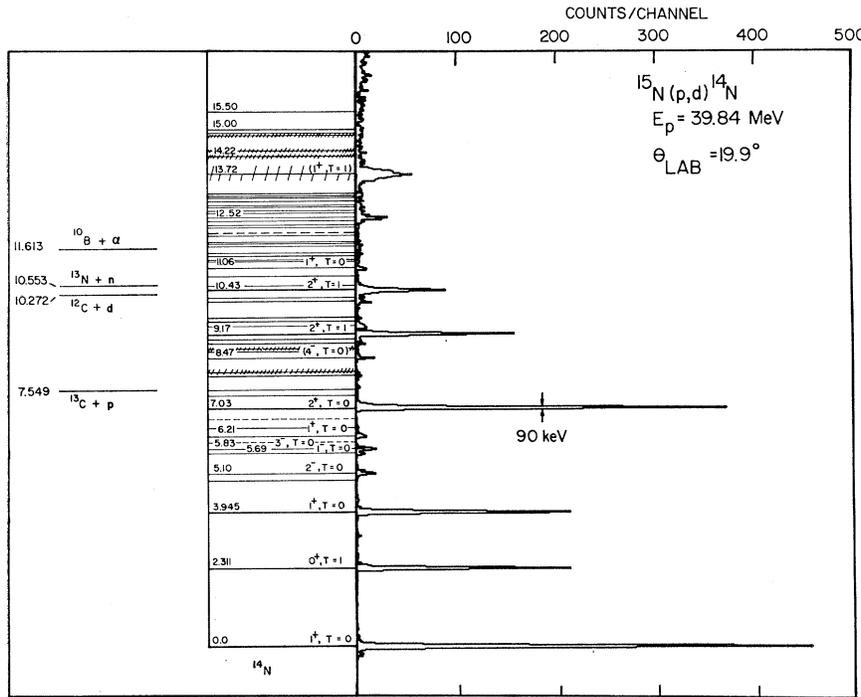
FIG. 3. Energy-level diagram of  $^{14}\text{N}$  displayed beside a deuteron energy spectrum from the  $^{15}\text{N}(p, d)^{14}\text{N}$  reaction for  $E_p = 39.84$  MeV and  $\theta_{\text{lab}} = 19.9^\circ$ .
