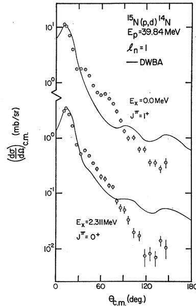
FIG. 7. DWBA calculations for the  $^{15}\text{N}(p, d)^{14}\text{N}$ ,  $E_p=39.84$  MeV,  $E_x=0.0$ - and 2.311-MeV angular distributions.
