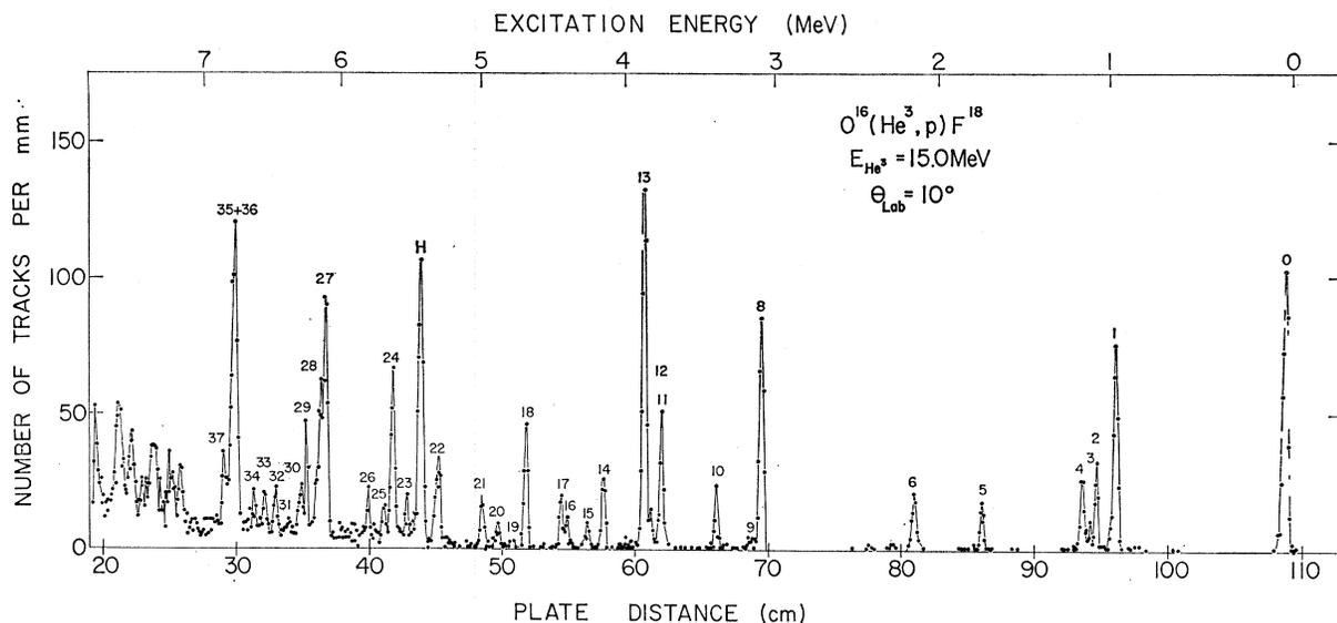
FIG. 3.  $O^{16}(He^3, p)F^{18}$  spectrum. Levels of  $F^{18}$  are numbered 0–37 and correspond to the excitation energies given in Table I. The group labeled *H* is recoil protons from the small hydrogen contaminant in the target gas.
