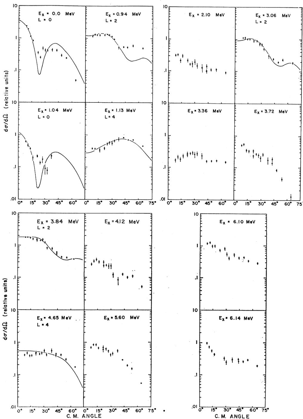
FIG. 4. Angular distributions of 14 proton groups leading to final states of  $F^{18}$  excited by the  $O^{16}(\text{He}^3, p)F^{18}$  reaction. The solid lines are DWBA calculations performed as explained in the text.
