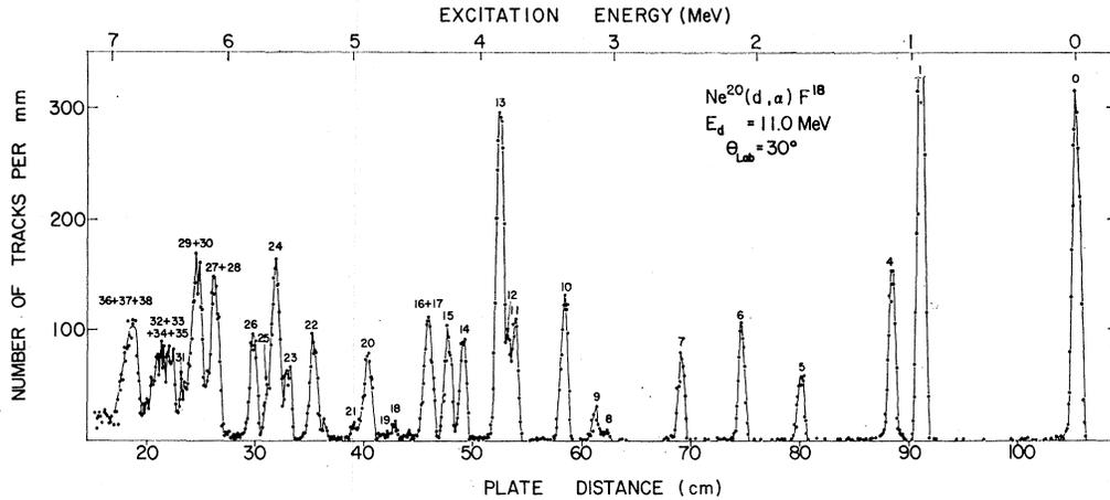
FIG. 5.  $Ne^{20}(d, \alpha)F^{18}$  spectrum. Levels of  $F^{18}$  are numbered 0 through 38 and correspond to the excitation energies given in Table I. Levels 2, 8, 18, 19, and 21 have been assigned  $T=1$ . Level 2 was not seen in this exposure.
