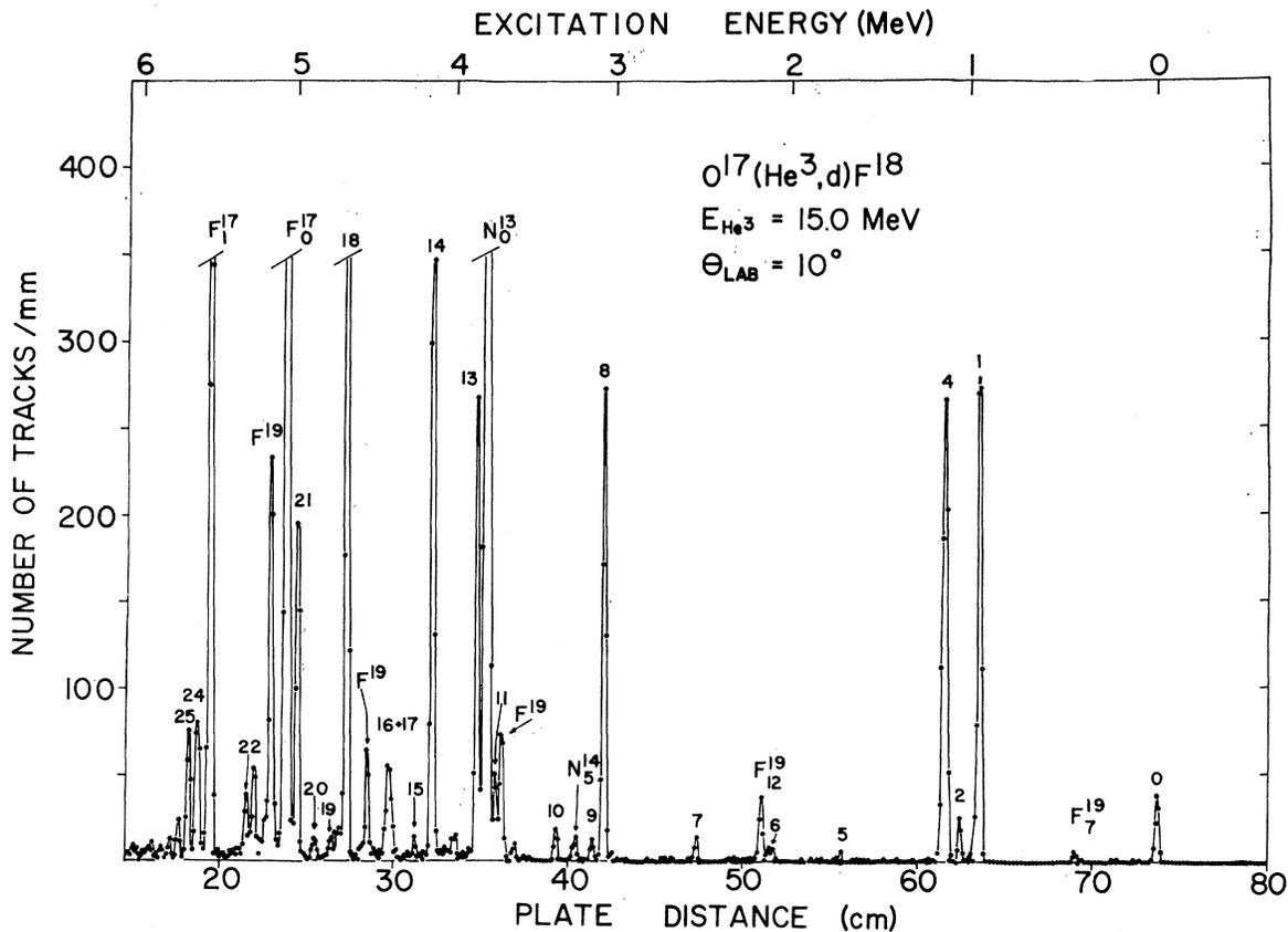
FIG. 1.  $O^{17}(He^3, d)F^{18}$  spectrum. Levels of  $F^{18}$  are numbered 0-25 and correspond to the excitation energies given in Table I. Impurity groups that could be definitely identified are indicated by the appropriate residual nucleus. Such groups arose from  $O^{18}$ ,  $O^{18}$ , and  $C^{12}$  contaminants in the target.
