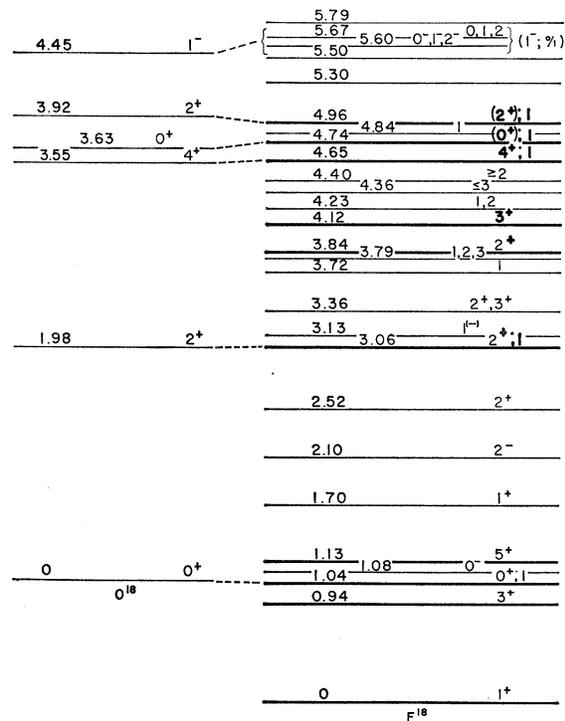
FIG. 6. Summary of information on  $F^{18}$  based on a synthesis of the results of the present study and the information given in Table I. Dark lines indicate states formed of  $(sd)^2$  configurations; new spin, parity, and isospin assignments made in this work are indicated in bold face. There is some evidence that the 3.72-MeV level is the  $1^+(sd)^2$  level predicted to lie at 3.77 MeV. The levels of  $O^{18}$  are also shown for comparison with the  $T=1$  states of  $F^{18}$ .
