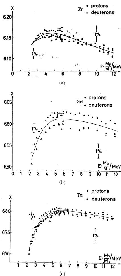
FIG. 1. Measured stopping powers of Zr, Gd, and Ta expressed by the reduced variable *X* defined by Eq. (2). The height of the arrows indicates the change in *X* caused by a 1% change in stopping power at the respective energies. *M<sub>p</sub>/M* is the ratio between proton mass and mass of incident particle (see text).
