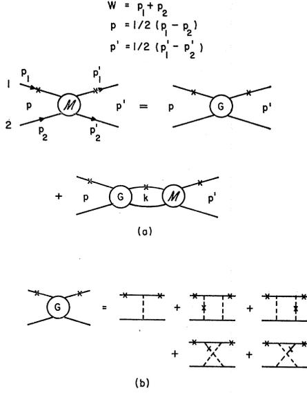
FIG. 3. Symbolic representation of the integral equation and potentials (up to two-boson-exchange terms). A cross on any particle line means that the particle is restricted to its mass shell.
