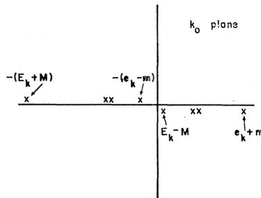
FIG. 5. Location of the singularities in the complex *k*<sub>0</sub> plane of the integrand of Eq. (3.20) for **p** = **p**' = 0.
