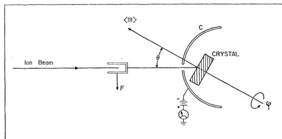
FIG. 2. A schematic diagram of the apparatus showing the mutual perpendicular rotations  $\theta$  and  $\varphi$  of the silicon crystal.
