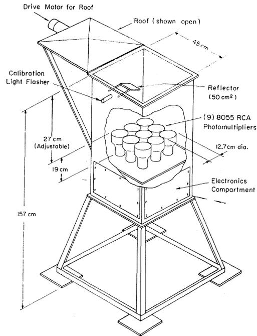
FIG. 2. Cutaway drawing of an individual CL detector.
