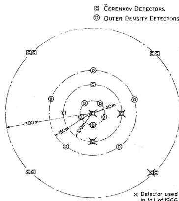
FIG. 1. Schematic map showing the locations of the outer detectors of the BASJE array and the locations of the CL detectors. The four CL detectors used during the 1966 operation are indicated.
