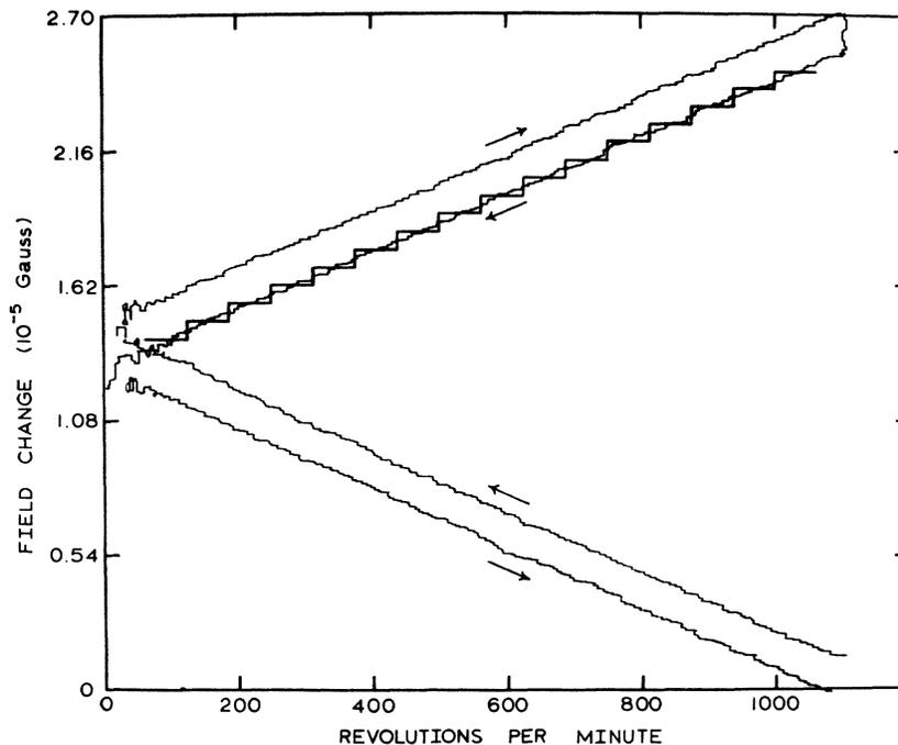
FIG. 3. Example of London-moment data. 6-mm tin single crystal rod, 1.20°K. The arrows indicate direction of speed change. The individual plots are spaced by changing the y-axis zero of reference. The steps that have been drawn in represent the postulated single-fluxoid steps (see text).
