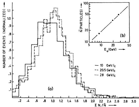
FIG. 2. Results of the Brookhaven measurements. (a) shows histograms of the number of events versus the energy deposit  $\sum N_i$  in the spectrometer.  $\sum N_i$  is expressed in units of its average,  $\bar{N}$ . The experimental results are for the three primary proton momenta indicated. (b) shows the dependence of  $\bar{N}$  on the primary kinetic energy  $E_0$ .
