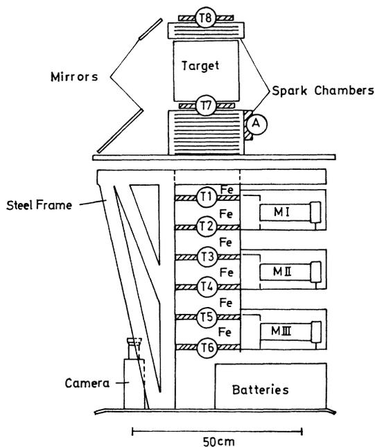
FIG. 1. Schematic drawing of the balloon instrument. Scintillation counter *A* is in anticoincidence, counters *T1*, . . . , *T8* record various trigger thresholds, and counters *MI*, *MII*, and *MIII* measure the cascade development in the ionization spectrometer.
