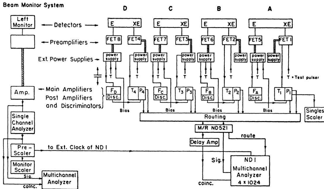
Fig. 2. Block diagram of a typical electronic network for use with position-sensitive counters A, B, C, and D. The circuit routes and stores the position $\times$ energy product (XE) without division of XE by E.
