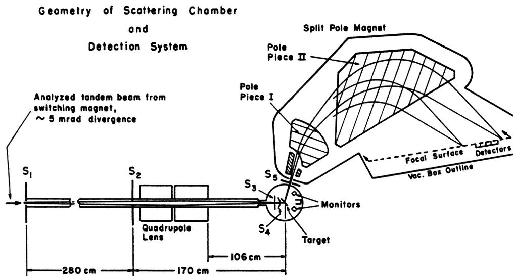
FIG. 1. Sketch of the experimental setup showing the incident beam path and the reaction product trajectories to the position detectors at the focal surface of the magnet.
