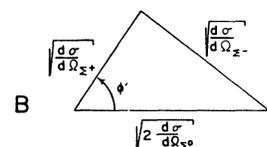
FIG. 1. Charge independence in strong interactions forces the reaction amplitudes for  $\Sigma K$  production to form the triangle (A) in the complex plane. Because the differential cross sections are the squares of amplitudes summed over spin states, the appropriate square roots of the cross sections must also form a closed triangle (B). This leads to three "triangle inequalities" among the cross sections.
