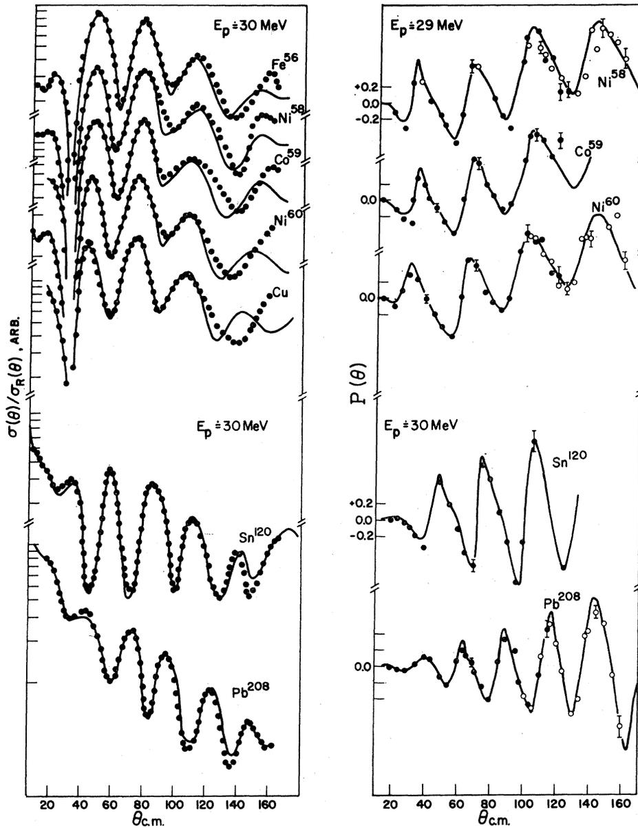
FIG. 11. Comparison of experimental cross-section and polarization data with the best-fit predictions for protons.  $E_p = 30$  MeV, ● (Ref. 27);  $E_p = 29$  MeV, ● (Ref. 28), ○ (Ref. 29).
