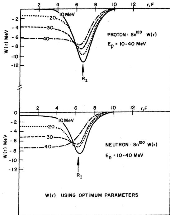
FIG. 13. Plots of the best-fit neutron and proton imaginary potentials found for  $\text{Sn}^{120}$ .
