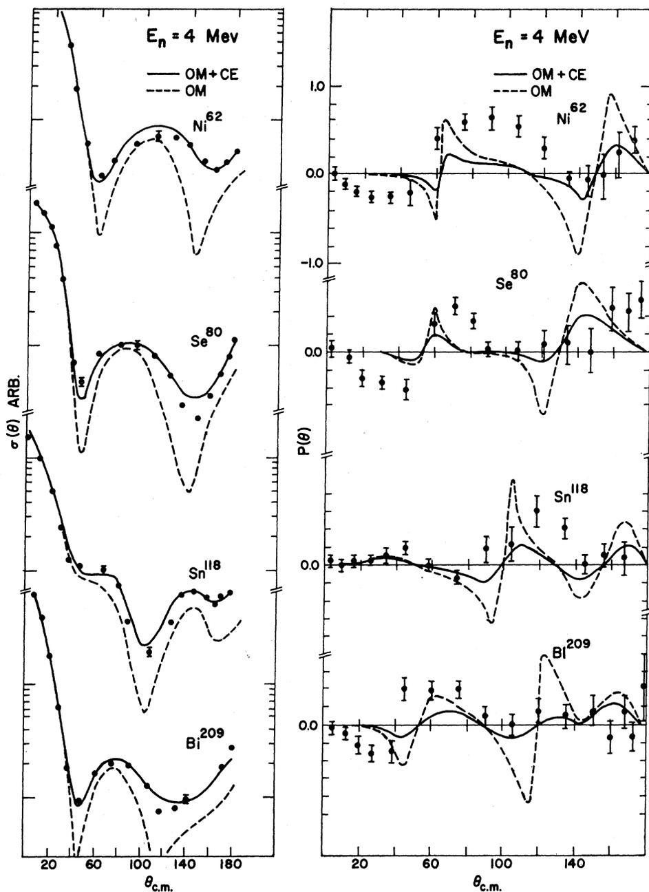
FIG. 17. Comparison of experimental cross-section and polarization data with the best-fit predictions for neutrons,  $E_n=4$  MeV (Ref. 49).
