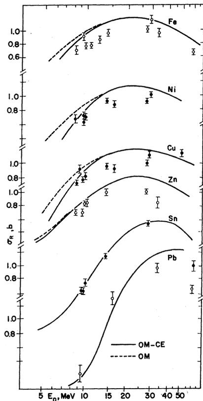
FIG. 4. Comparison of the reaction cross-section predictions with experimental values using the proton best-fit parameters (Refs. 11-16 and 42, 43).
