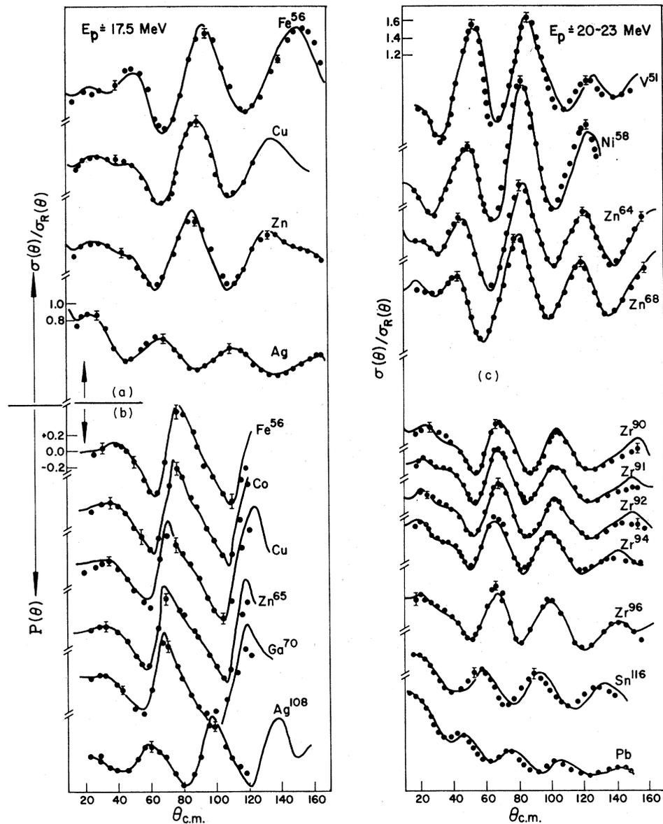
FIG 10. Comparison of experimental cross-section and polarization data with the best-fit predictions for protons,  $E_p = 17-23$  MeV. (a) Ref. 23, (b) Ref. 24, and (c) Refs. 25, 26.
