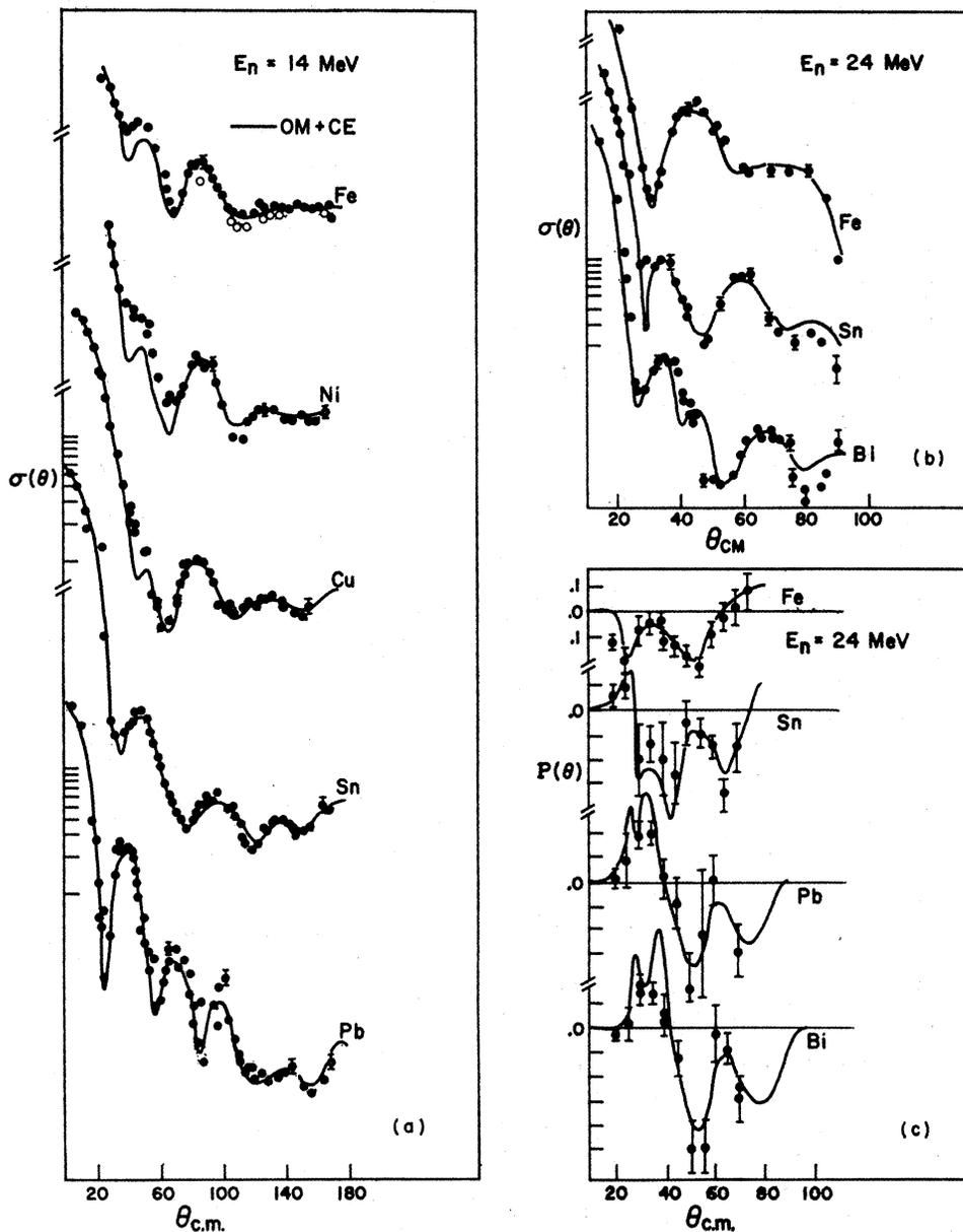
FIG. 18. Comparison of experimental cross-section and polarization data with the best-fit prediction for neutrons,  $E_n = 14$  and 24 MeV. (a) Refs. 36, 37, (b) Ref. 38, and (c) Ref. 39.
