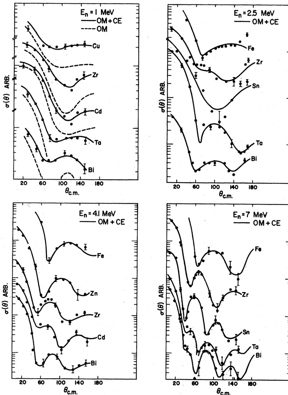
FIG. 16. Comparison of experimental cross-section data with the best-fit predictions for neutrons,  $E_n = 1-7$  MeV (Ref. 35).
