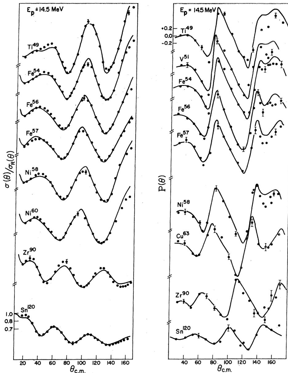
Fig 9. Comparison of experimental cross-section and polarization data with the best-fit predictions for protons,  $E_p = 14.5$  MeV.  $\sigma(\theta)/\sigma_R(\theta)$  (Ref. 22) and  $P(\theta)$  (Ref. 21).
