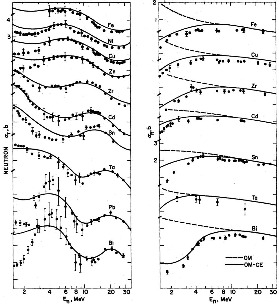
FIG. 14. Comparison of the total and reaction cross-section predictions with experimental values using the neutron best-fit parameters (Ref. 33).
