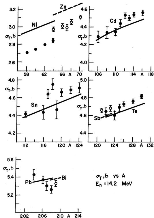
FIG. 15. Comparison of the total cross-section predictions for isotopic sequences (with experimental values using the neutron best-fit parameters (Ref. 34)).
