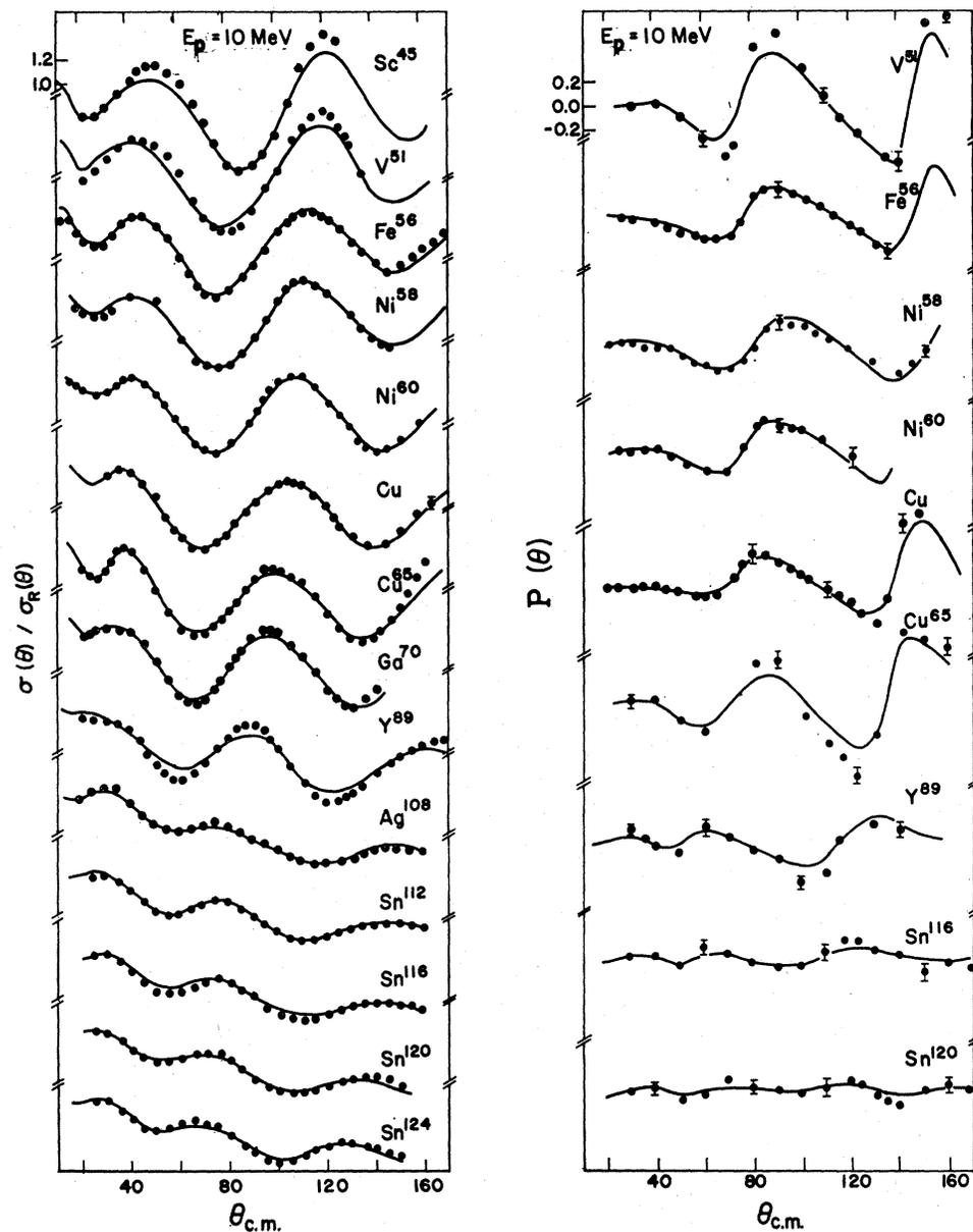
FIG. 8. Comparison of experimental cross-section data with the best-fit predictions for protons,  $E_p=10$  MeV.  $\sigma(\theta)/\sigma_R(\theta)$  (Refs. 17-19, 44) and  $P(\theta)$  (Refs. 20, 21).
