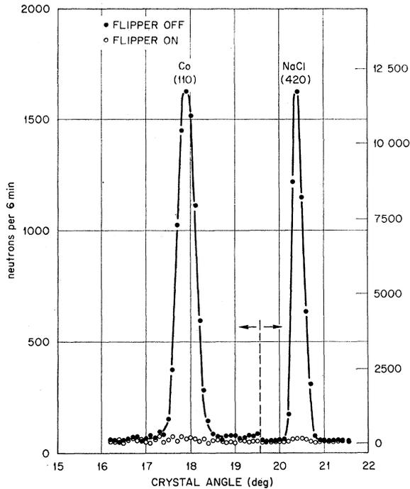
FIG. 1. Polarization analysis of the Co (110) and NaCl (420) reflections.  $|\hat{K} \cdot \hat{\eta}(0)| = 1$ ,  $|\hat{K} \cdot \hat{z}| = 1$ .
