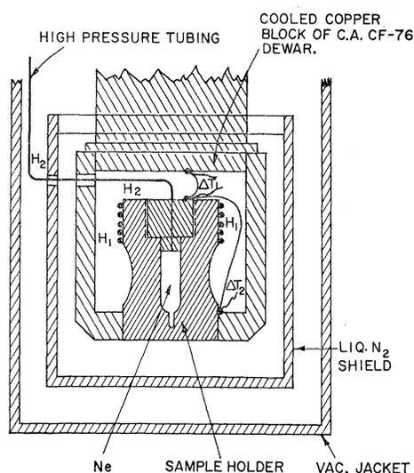
Fig. 1. Cell used in preparation of neon crystals at high pressure.
