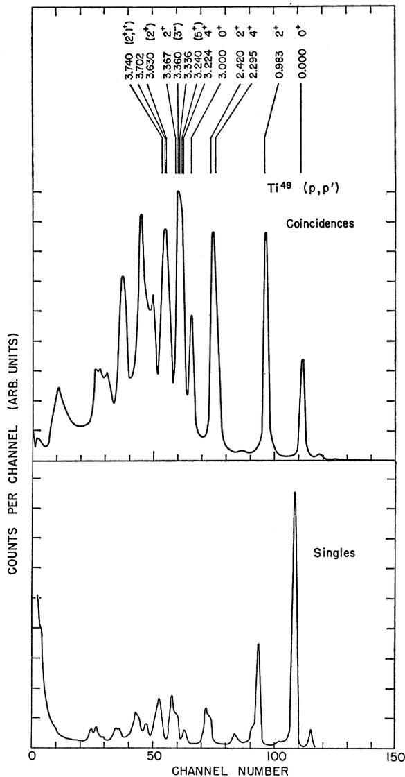
FIG. 1. Spectrum of protons inelastically scattered from  $Ti^{48}$  at a lab angle of approximately  $160^\circ$  (see text) both with and without a coincidence with a  $\gamma$  ray.
