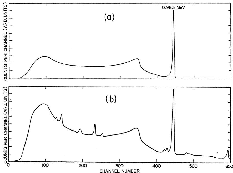
FIG. 4. (a) Spectrum of  $\gamma$  rays in coincidence with protons from group "A" of Fig. 1. (b) Spectrum of  $\gamma$  rays in coincidence with protons of any energy above 0.5 MeV.
