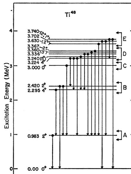
FIG. 2. Decay scheme for  $Ti^{48}$ . Energies of levels are based on a comparison of the results of this experiment with results reported in Refs. 4 and 5.
