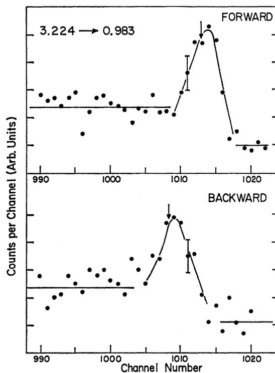
FIG. 6. Doppler-shift data for the 3.224-MeV  $4^+$  to 0.9833-MeV  $2^+$  transition, obtained from the  $\gamma$ -ray events in coincidence with protons from group "D" of Fig. 1. The arrows indicate the computed positions of the peak centroids. A tail on the low-energy side of the peak causes the mean to not correspond to the maximum.
