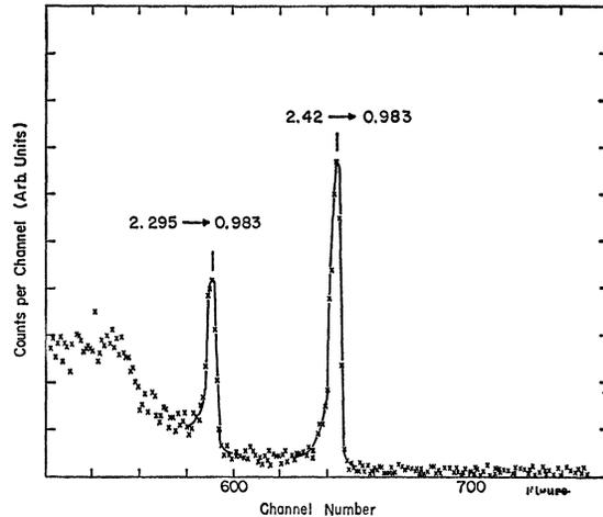
FIG. 3. Spectrum of  $\gamma$  rays in coincidence with protons of any energy above 0.5 MeV, for the region around  $E_\gamma = 1.5$  MeV.
