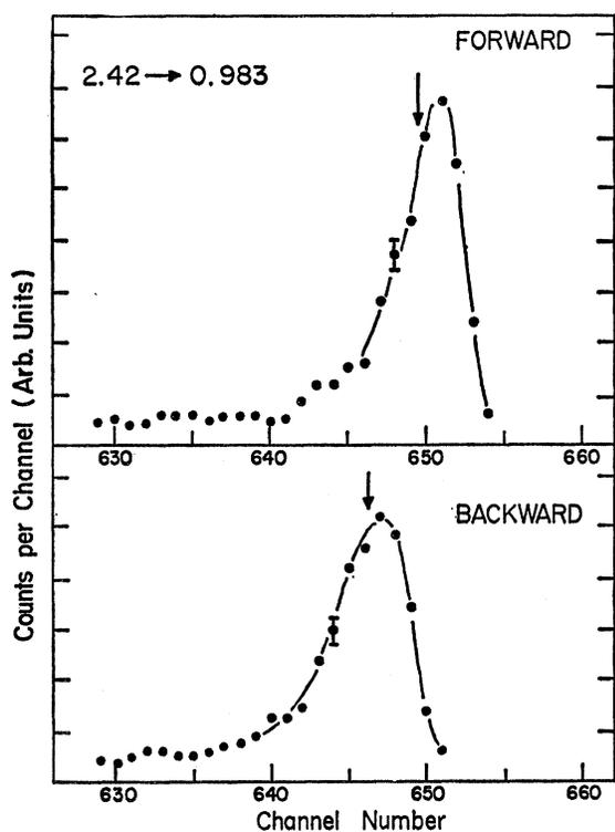
FIG. 5. Doppler-shift data for the 2.420-MeV  $2^+$  to 0.9833-MeV  $2^+$  transition, obtained from the  $\gamma$ -ray events in coincidence with protons from group "B" of Fig. 1. The arrows indicate the computed positions of the peak centroids. A tail on the low-energy side of the peak causes the mean to not correspond to the maximum.
