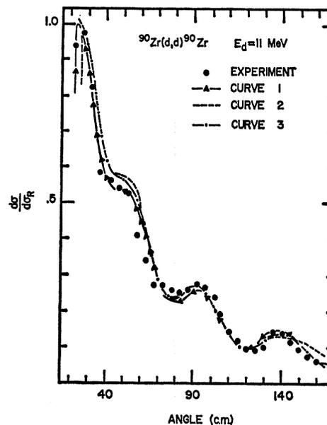
FIG. 4.  $^{90}\text{Zr}(d, d)^{90}\text{Zr}$  experimental cross sections and optical-model fit at  $E_d = 11$  MeV.
