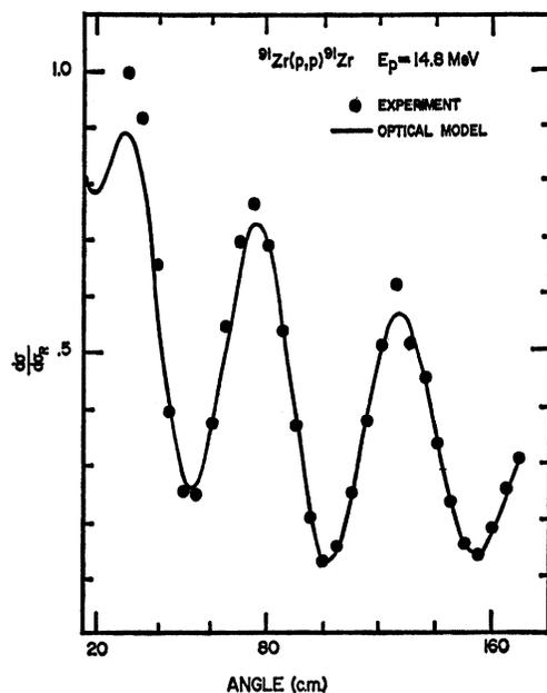
FIG. 7.  $^{91}\text{Zr}(p, p)^{91}\text{Zr}$  experimental cross sections and optical-model fit at  $E_p = 14.8$  MeV.
