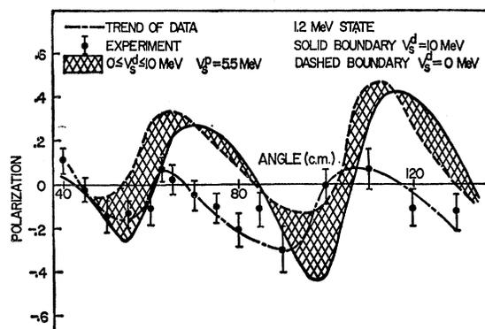
FIG. 11.  $^{90}\text{Zr}(d, p)^{91}\text{Zr}^*$  (1.2 MeV) experimental polarizations compared with the DWBA predictions allowing the deuteron spin-orbit potential to vary between 0 and 10 MeV.
