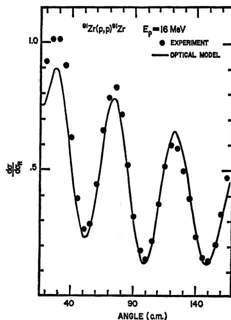
FIG. 5.  $^{91}\text{Zr}(p, p)^{91}\text{Zr}$  experimental cross sections and optical-model fit at  $E_p = 16$  MeV.
