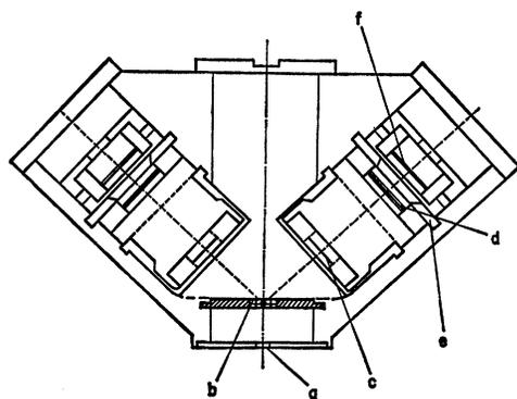
FIG. 2. The carbon-foil polarimeter: g, e collimators; b, carbon foil; c, d, and f, detectors.
