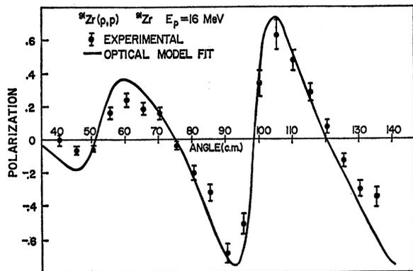
FIG. 6.  $^{91}\text{Zr}(p, p)^{91}\text{Zr}$  experimental polarizations and optical-model fit at  $E_p = 16$  MeV.
