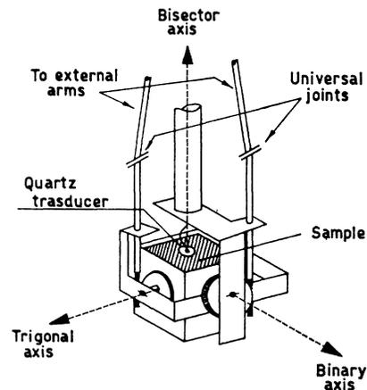
FIG. 1. Sample arrangement.
