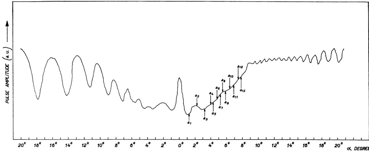
FIG. 8. Echo-pulse amplitude as a function of the angle  $\alpha$  between the trigonal axis and the magnetic field direction. The magnetic field lies in the trigonal-bisector plane, and the sound wave vector is along the bisector axis. The magnetic field strength is 5 kG.
