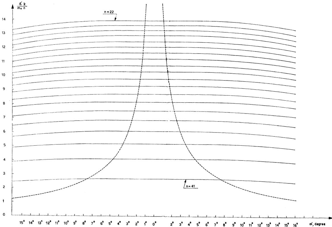
FIG. 12. Spacing of hole Landau levels in  $k$  space as a function of the angle  $\alpha$  between magnetic field direction and trigonal axis (solid lines). Dashed line refers to  $k_H$  as given by Eq. (1).
