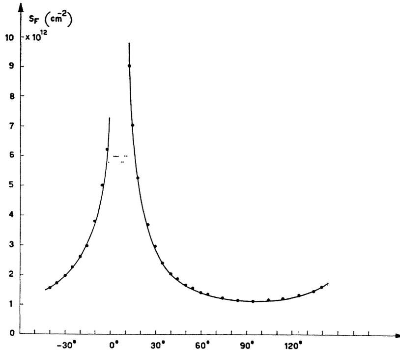
FIG. 3. Fermi-surface cross sections for magnetic field directions in the trigonal-bisector plane. Angles are measured from the trigonal axis.
