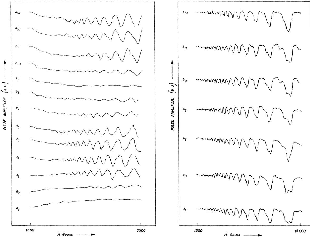
Fig. 9. Echo-pulse amplitude versus magnetic field intensity. The magnetic field lies in the trigonal-bisector plane. Left-hand side: sound wave vector along the bisector axis (see Fig. 8). Right-hand side: sound wave vector along the trigonal axis.
