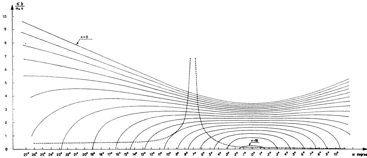
FIG. 11. Spacing of electron Landau levels in  $k$  space [Eq. (2)] as a function of the angle  $\alpha$  between the magnetic field direction and trigonal axis (solid lines). Dashed line refers to  $k_H$  as given by Eq. (1).
