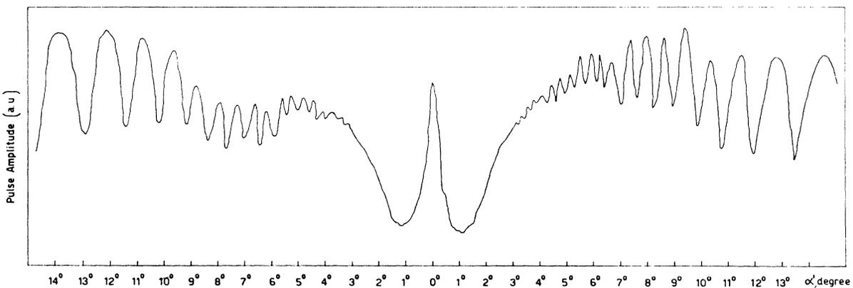
Fig. 10. Echo-pulse amplitude versus the angle  $\alpha'$  between the binary axis and the magnetic field direction. The magnetic field vector lies in the bisector-binary plane, and the sound wave vector is along the bisector axis. The magnetic field strength is 5 kG.
