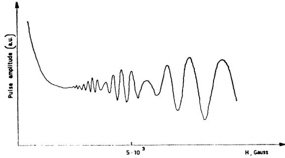
FIG. 6. Echo-pulse amplitude versus magnetic field intensity. The field direction corresponds to the point A in Fig. 5.
