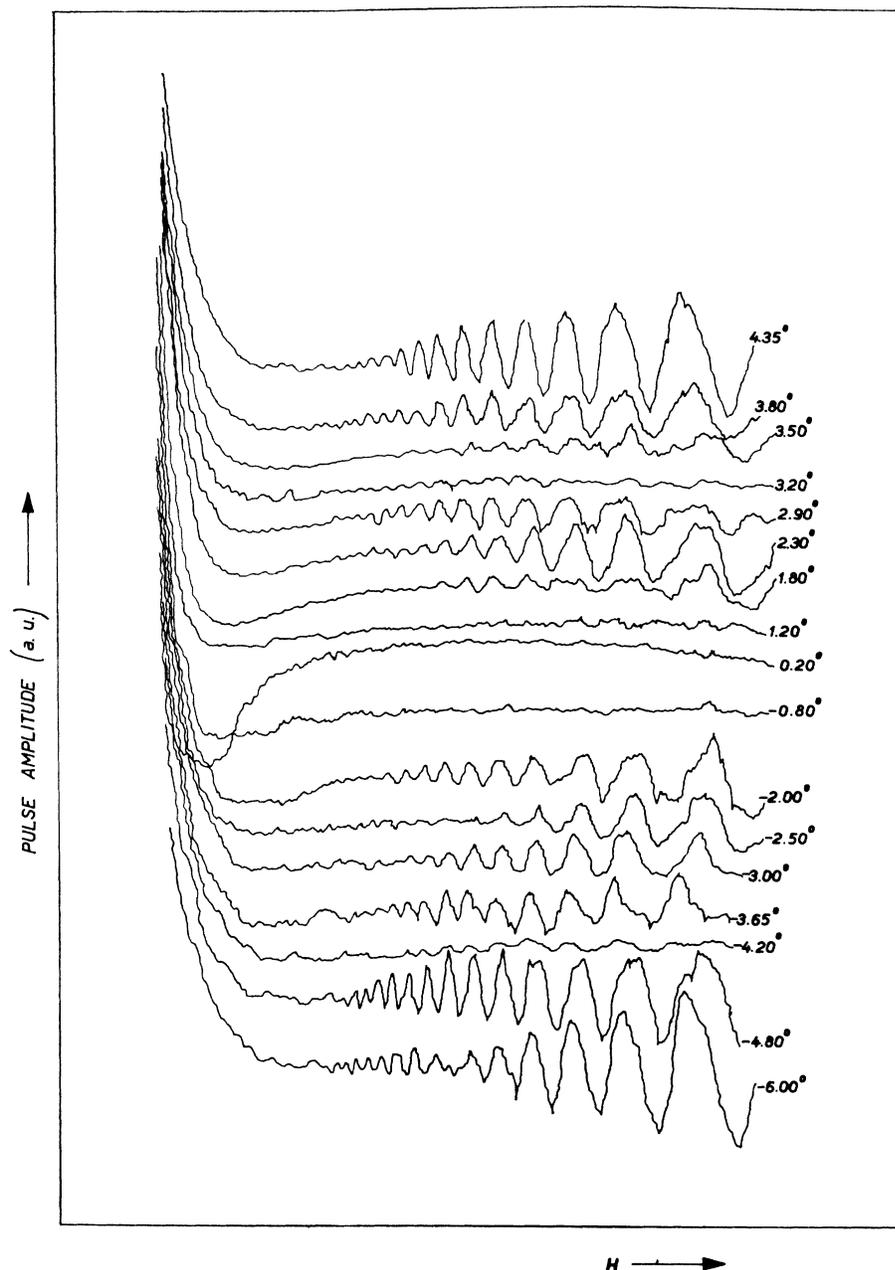
FIG. 7. Echo-pulse amplitude as a function of magnetic field intensity for various orientations of the magnetic field in the trigonal-binary plane; the sound wave vector lies along the binary axis.
