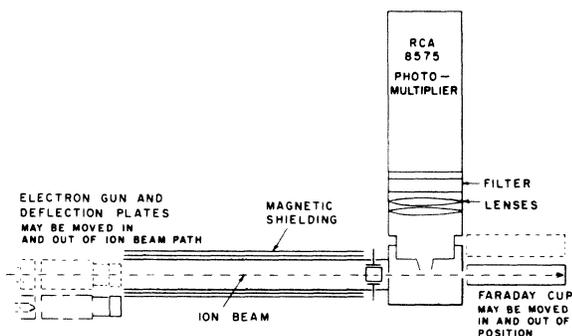
FIG. 1. Experimental arrangement for the study of excitation of 3914 Å light in collisions of ions with  $N_2$ . The removable electron gun is used alternatively with the ion beam and a comparison of the signals observed yields the ratio of the cross sections for electron-impact and ion-impact excitation.
