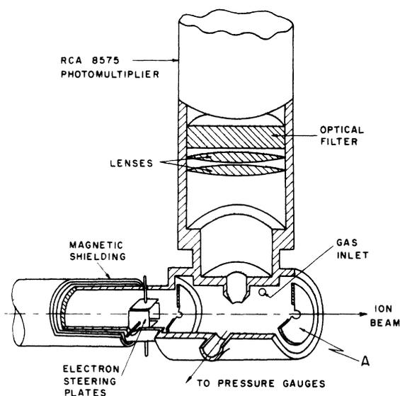
FIG. 2. Details of the collision chamber and optics used in studying excitation of 3914 Å radiation.
