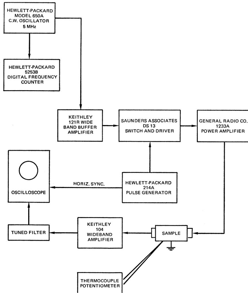
FIG. 1. Schematic circuit diagram.
