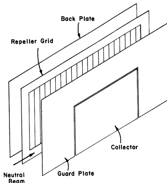
FIG. 3. Ionization chamber.
