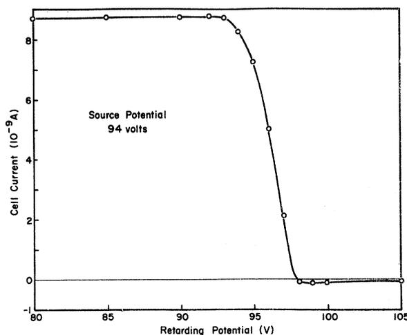
FIG. 2. Energy distribution of proton beam in charge transfer cell measured by retardation method.
