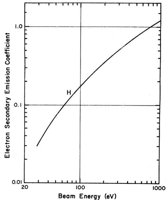
FIG. 12. Secondary-electron-emission coefficient for impact of hydrogen atoms on a copper surface under an angle of 45 deg.
