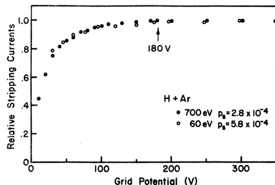
FIG. 5. Collection efficiency of stripping cell as function of extraction voltage.
