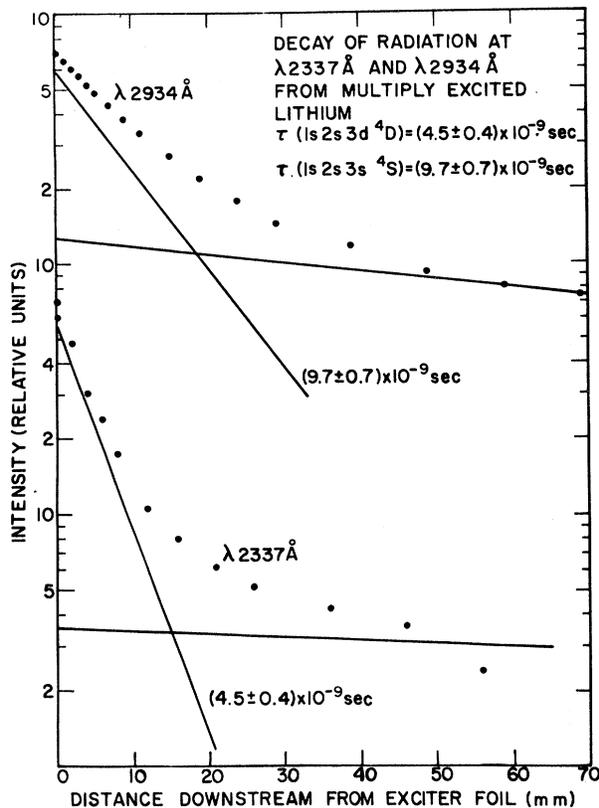
FIG. 3. The results of five independent measurements of the radiation at  $\lambda 2337 \text{ \AA}$  ( $1s2s3d^4D \rightarrow 1s2s2p^4P$ ) and  $\lambda 2934 \text{ \AA}$  ( $1s2s3s^4S \rightarrow 1s2s2p^4P$ ) from Li I as a function of distance  $x$  downstream from the exciter foil. The decays of both excited levels are affected by cascades.
