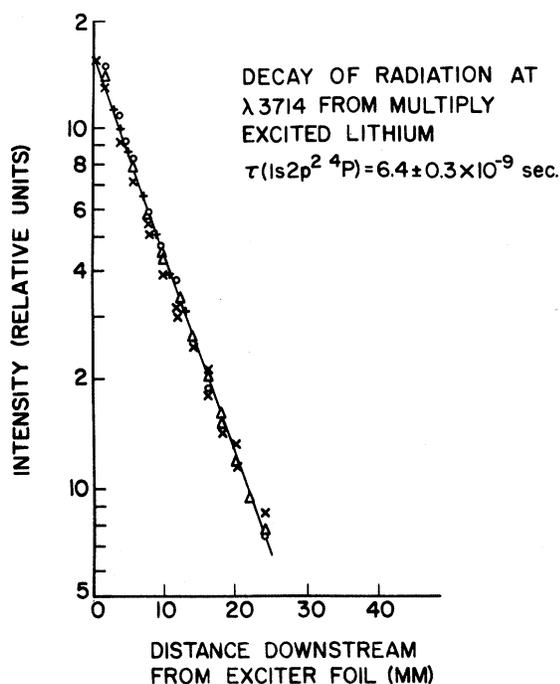
FIG. 2. The result of seven independent measurements of the intensity of radiation at  $\lambda 3714 \text{ \AA}$  ( $1s2p^2 4P \rightarrow 1s2s2p^4 P$ ) from Li I as a function of distance  $x$  downstream from the exciter foil. The slope of the curve yields a mean life  $\tau = (6.4 \pm 0.3) \times 10^{-9}$  sec for the  $1s2p^2 4P$  level.
