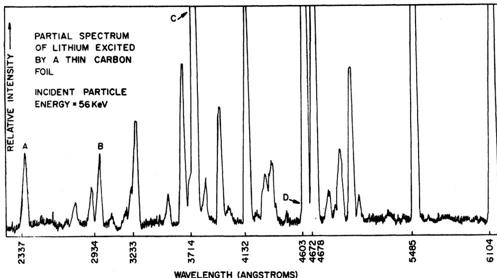
FIG. 1. Part of a spectral scan obtained from beam-foil-excited lithium atoms. The signals assigned to the decay of doubly excited levels are labeled A, B, C, and D.
