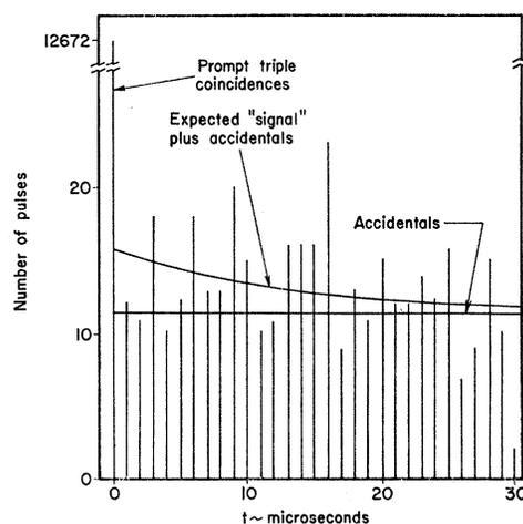
FIG. 6. "Neutron time distribution—number of pulses versus time." The expected "signal" time distribution is determined from the neutron capture time in the Gd solution.
