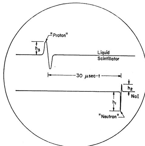
FIG. 2. Oscilloscope trace showing data output. The upper trace is due to the "proton" pulse, the lower to the "neutron" pulse. The pulses from the crystals were coded and mixed to have opposite polarities and be delayed by about 1  $\mu\text{-sec}$  relative to each other.  $h_1$  and  $h_2$  are the pulse heights produced by crystals 1 and 2 respectively and  $h_3$  is the pulse height produced by the liquid scintillator.
