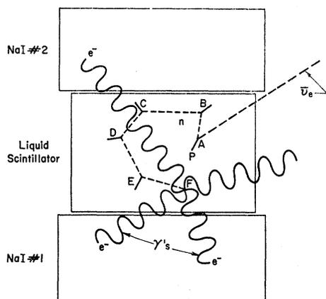
FIG. 1. Hypothetical  $\bar{\nu}_e$  disintegration of a deuteron. Reactor neutrino comes from the right and strikes deuteron at A, disintegrating it. The neutron and proton carry off kinetic energy. The neutron strikes nuclei at B, C, D, and E before becoming thermal, after which it wanders around until it is captured at F by a gadolinium nucleus. On the average four  $\gamma$ 's are emitted. The  $\gamma$ 's then are detected by the NaI crystals.
