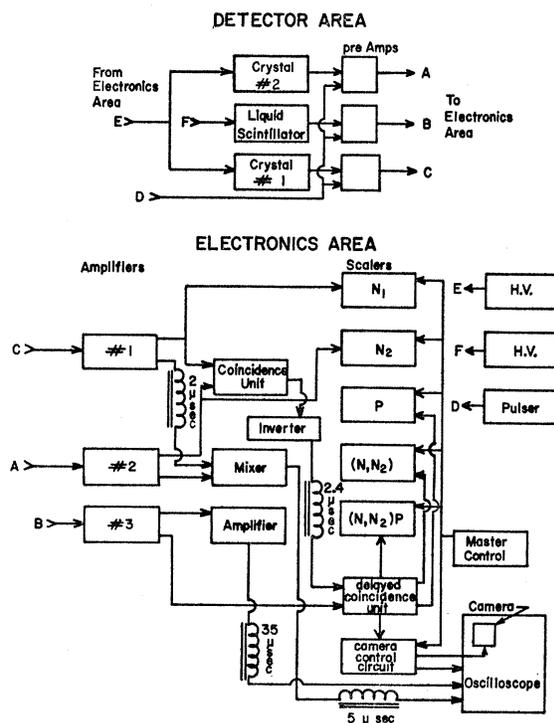
FIG. 4. Electronics block diagram.
