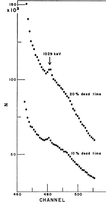
FIG. 2. The portion of the  $^{200}\text{Tl}$   $\gamma$ -ray spectrum in the vicinity of 1029 keV obtained at two different count rates.
