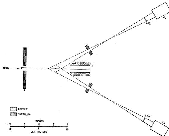
FIG. 1. Scale drawing of the scattering geometry as seen from above. The beam outline represents the region of half-maximum intensity of the first run.
