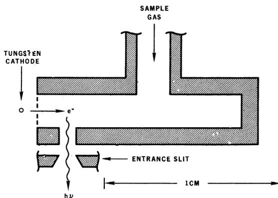
FIG. 2. Pulsed electron, hollow anode source.
