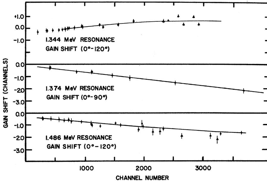
FIG. 2. Plots of the discrete gain changes which occurred in moving the detector from one angle to the next in the Doppler-shift measurements at the  $E_p = 1.344$ , 1.374-, and 1.486-MeV resonances. Solid circles represent data obtained from  $\text{Co}^{66}$  lines; triangles are points obtained from  $\gamma$  rays which decayed from the resonance state, corrected for full Doppler shift.
