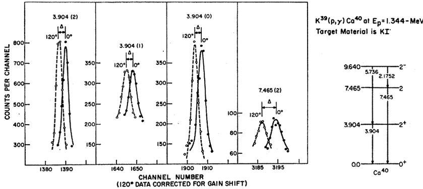
FIG. 5. Experimental results of the Doppler-shift measurements at the  $E_p=1.344$ -MeV resonance using a KI target. The lifetimes of the 7.465- and 3.904-MeV levels populated in the decay of the resonance excited state are inferred from the attenuated Doppler shifts measured at  $120^\circ$  and  $0^\circ$ .
