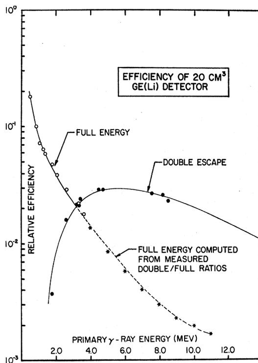
FIG. 1. The relative photopeak and double-escape-peak efficiency curves. The projected full-energy curve was obtained from the experimentally determined ratio of the photopeak intensity to double-escape-peak intensity. Points below 3.5 MeV were obtained with a  $Co^{56}$  source. Relative double-escape efficiency above this energy was obtained from  $Al^{27}(p,\gamma)Si^{28}$  and  $K^{39}(p,\gamma)Ca^{40}$  intensity measurements.
