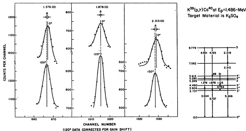
Fig. 6. Experimental results of the Doppler-shift measurements at the  $E_p=1.486$ -MeV resonance using a  $K_2SO_4$  target. The lifetimes of the 5.280-, 5.615-, and 7.562-MeV levels are inferred from the attenuated Doppler shifts measured at  $120^\circ$  and  $0^\circ$ .
