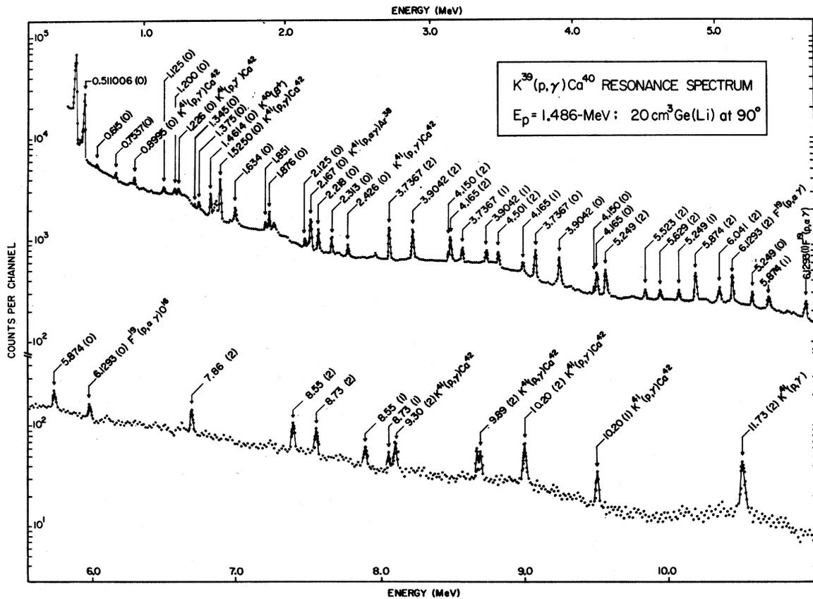
FIG. 3. The  $E_p = 1.486$ -MeV resonance spectrum recorded at  $90^\circ$  with a  $20\text{-cm}^3$   $\text{Ge(Li)}$  detector. The  $\text{K}^{41}(p,\gamma)\text{Ca}^{42}$  peaks are due to the  $\text{K}^{41}$  present in the natural potassium-iodide target. Other contaminant lines are labeled on the figure.
