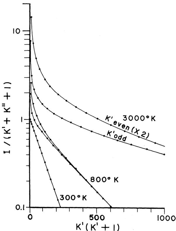
FIG. 3. Computed plot of  $\ln(I/K')$  versus  $K'(K'+1)$  at various rotational temperatures for the  $N_2^+$  first negative (0,0) band. Intensities of points corresponding to  $K'$  even lines have been multiplied by 2.
