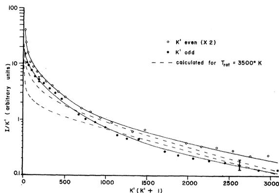
FIG. 8. Plot of  $\ln(I/K')$  versus  $K'(K'+1)$  taken from spectra of the  $N_2^+$  first negative (0,0) band excited by 0.4-keV  $H_2^+$ . The intensities of the lines of even  $K'$  have been multiplied by 2. The calculated curve for  $T_{rot} = 3500^\circ K$  is included for comparison. The reproducibility of the data is indicated by the error bars at each end of the plot.
