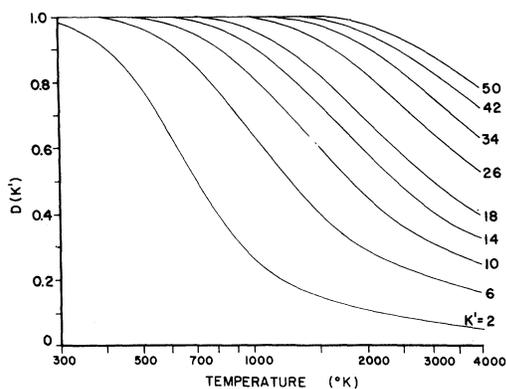
FIG. 4. Computed ratio of  $R$ -branch line intensity to total line intensity including  $P$ -branch overlap versus rotational temperature for  $\text{N}_2^+$  first negative  $(0,0)$  band lines with even  $K'$ . These curves cannot be used for the  $(0,1)$  band (see text).
