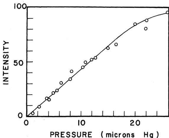
FIG. 2. Intensity of the  $N_2^+$  first negative system (0,0) band head ( $\lambda$  3914 Å) versus collision-chamber pressure. The 1000-eV  $H_2^+$  ion current was constant at 30  $\mu$ A during these measurements.
