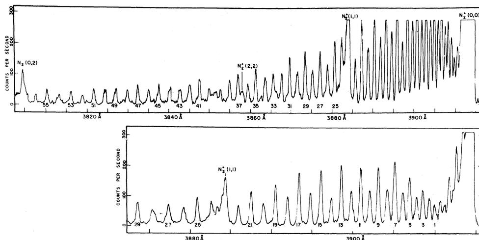
FIG. 6. Typical spectra of the  $\text{N}_2^+$  first negative  $(0,0)$  band ( $\lambda 3914 \text{ \AA}$ ) excited by a  $46\text{-}\mu\text{A}$  beam of  $1000\text{-eV H}_2^+$ . The pressure in the collision chamber was  $5.5 \mu \text{ Hg}$ . The upper spectrum was taken with a spectrometer-slit width of  $70 \mu$ , while the lower expanded trace was taken with a  $30\text{-}\mu$  slit. The effects of perturbations appear at  $K' = 14$  and  $K' = 39$  (see text).
