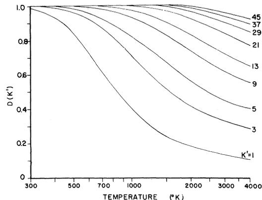
FIG. 5. Computed ratio of  $R$ -branch line intensity to total line intensity including  $P$ -branch overlap versus rotational temperature for  $\text{N}_2^+$  first negative  $(0,0)$  band lines with odd  $K'$ . These curves cannot be used for the  $(0,1)$  band (see text).
