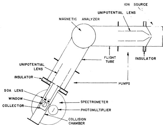
FIG. 1. Schematic diagram of the apparatus. The flight-tube section was maintained at  $-10$  kV. The ion beam was decelerated with the SOA lens.
