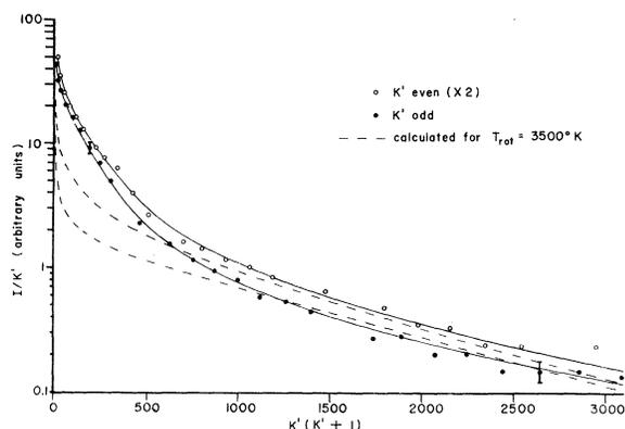
FIG. 7. Plot of  $\ln(I/K')$  versus  $K'(K'+1)$  taken from spectra of the  $N_2^+$  first negative (0,0) band excited by 3.0-keV  $H_2^+$ . The intensities of the lines of even  $K'$  have been multiplied by 2. The calculated curve for  $T_{rot} = 3500^\circ K$  is included for comparison. The reproducibility of the data is indicated by the error bars at each end of the plot.
