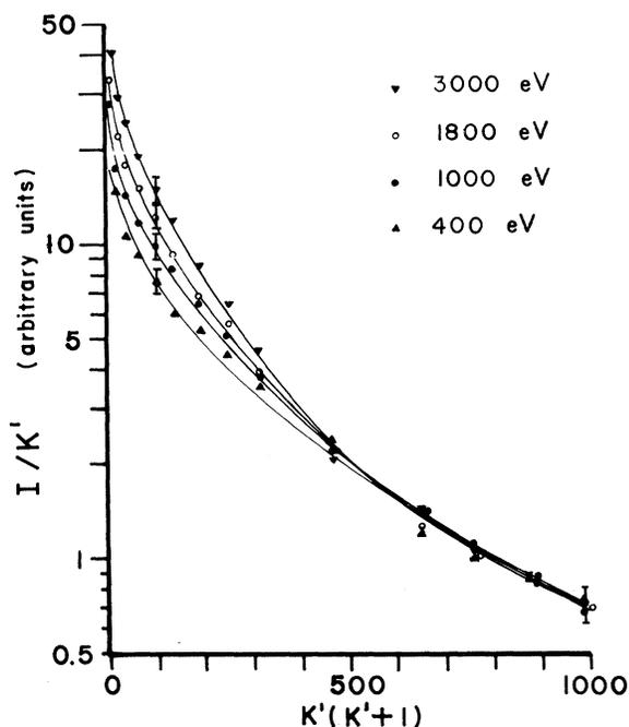
FIG. 9. Plots of  $\ln(I/K')$  versus  $K'(K'+1)$  taken from spectra of the  $N_2^+$  first negative (0,0) band excited by 0.4-, 1.0-, 1.8-, and 3.0-keV  $H_2^+$  on  $N_2$ . Only the lines with odd  $K'$  have been included. This figure illustrates the systematic change in curvature for low  $K'$  with projectile-ion energy. The curves have been normalized to coincide for  $K'(K'+1) > 1000$ . The reproducibility of the data is indicated by the error bars at each end of the plots.
