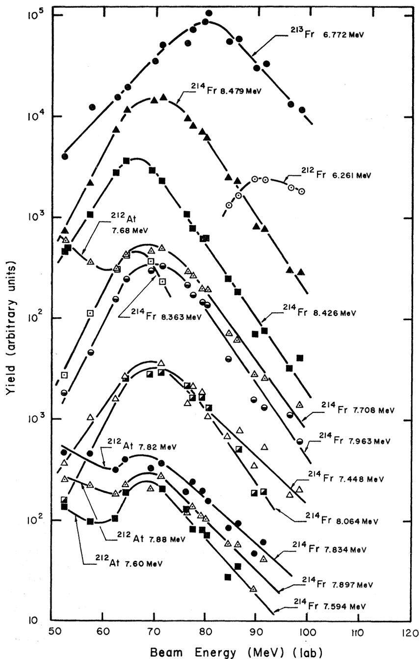
FIG. 2. Excitation functions for the  $\alpha$  groups of  $^{214}\text{Fr}$ ,  $^{213}\text{Fr}$ , and  $^{212}\text{Fr}$  produced in  $^{208}\text{Pb} + ^{11}\text{B}$  bombardments.
