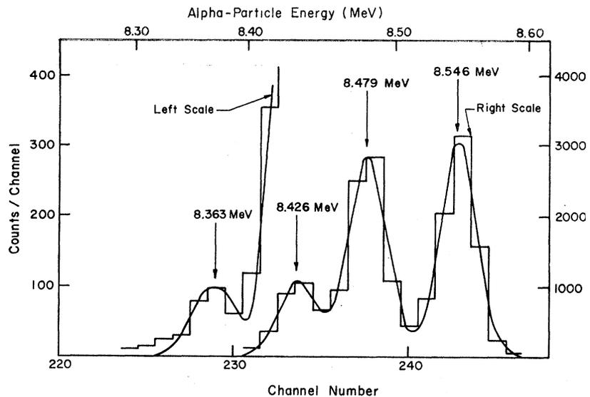
$^{214}\text{Ra}$  spectrum a value of  $0.059 \pm 0.004\%$  was obtained for the EC branch of  $^{214}\text{Ra}$ . A value of  $0.09 \pm 0.03\%$  has recently been obtained by Valli and co-workers.<sup>5</sup>
