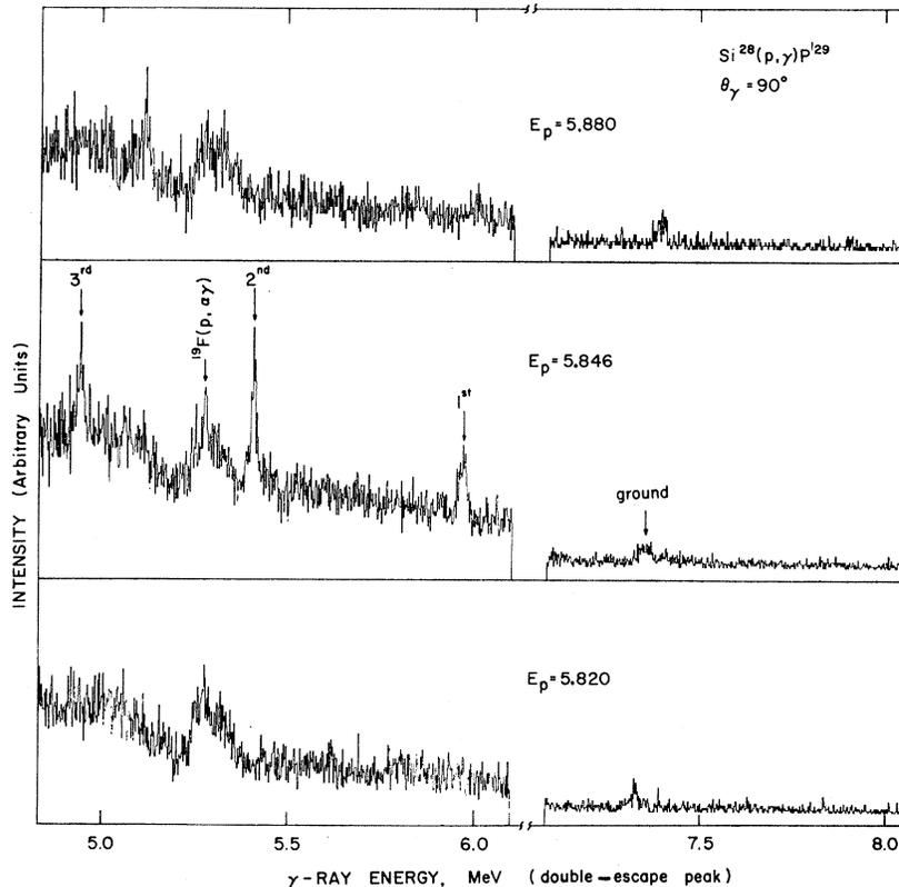
FIG. 4.  $\gamma$ -ray spectra taken on and off the 5.833-MeV resonance in Si<sup>28</sup>+ $p$ . The resonance spectrum was measured at a proton energy at which the yield was at a maximum for a target thick in terms of the energy spread of the system. The Ge(Li) detector was at 90° to the incident beam.
