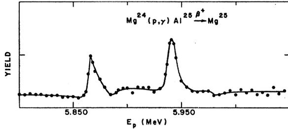
FIG. 1. Yield curve of  $Al^{25}$  activity resulting from the capture of protons by  $Mg^{24}$ .
