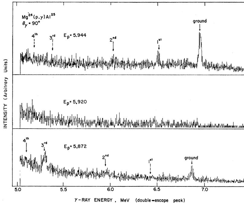
FIG. 2.  $\gamma$ -ray spectra taken on the 5.864- and 5.936-MeV resonances and at an off-resonance energy in  $\text{Mg}^{24}+p$ . Each resonance spectrum was measured at a proton energy at which the yield was at a maximum for a target thick in terms of the energy spread of the system. The Ge(Li) detector was at  $90^\circ$  to the incident beam.
