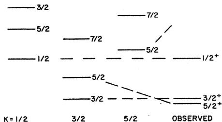
FIG. 7. Approximate unperturbed positions of the levels in the various  $T = \frac{3}{2}$  bands (solid lines) with the postulated shifting of the  $\frac{5}{2}^+$  levels (dotted lines) as a result of their mutual repulsion.
