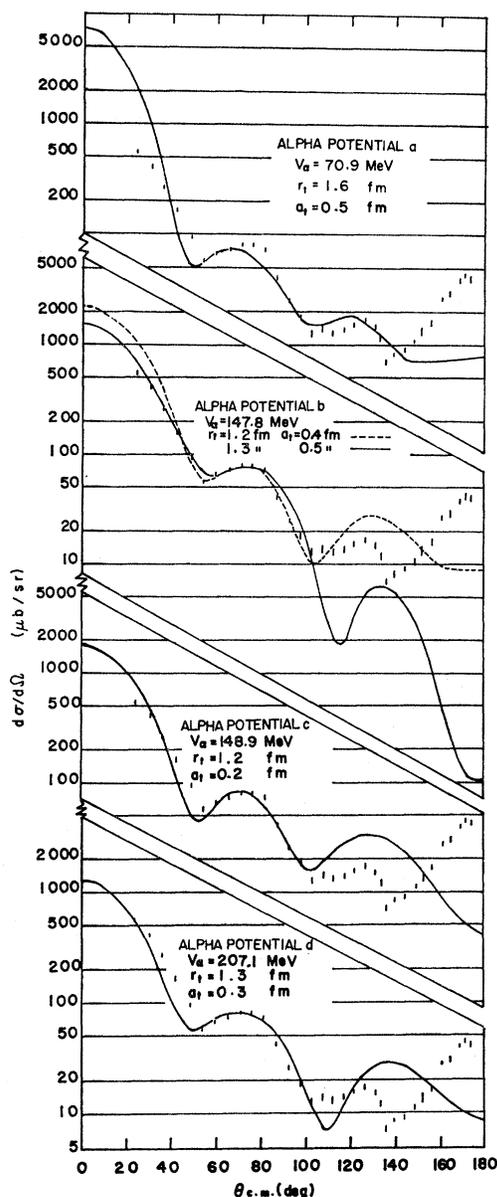
FIG. 2. DWBA fits to the reaction  $C^{12}(p, \alpha)B^9$  at 44.5 MeV. The triton potentials that best fit the forward part of the angular distribution are shown for each of the  $\alpha$  optical potentials of Table I. The  $LS$  spectroscopic factor of 1.498 has been included in the theoretical curves.
