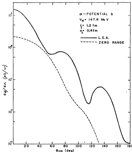
Fig. 3. The effect of the finite-range corrections on the angular distribution. The  $\alpha$  potential corresponds to solution (b) of Table I and the triton potential had values of  $r_t = 1.2$  fm and  $a_t = 0.4$  fm, for both curves.
