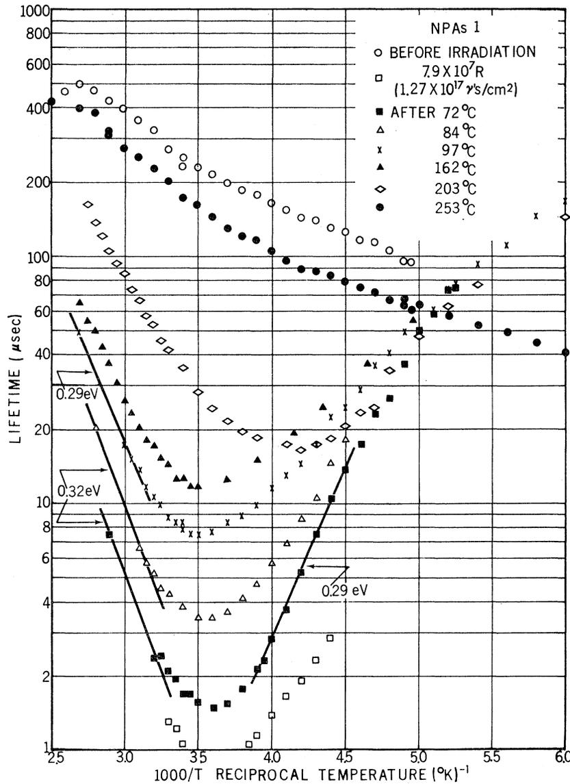
FIG. 7. The dependence of low-excess-density lifetime on temperature for NPAs 1.0 following  $\gamma$  irradiation and successive anneals.
