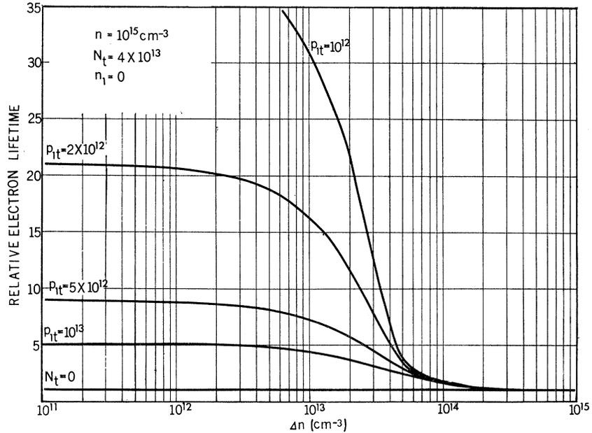
FIG. 3. Examples in which it is assumed that  $c_n > c_p$ , and again the recombination centers and traps are below the Fermi level. The behavior is similar if the recombination centers are above the Fermi level, except that there is an additional decrease in  $\tau$  for  $\Delta n \gtrsim n$ .
