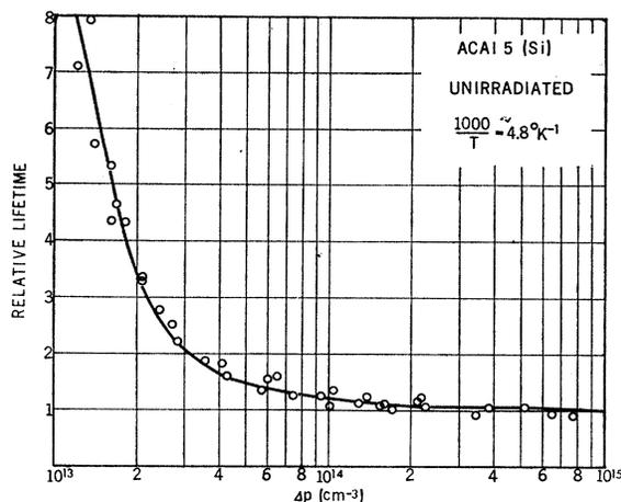
FIG. 6. The dependence of lifetime on excess density for a  $p$ -type (Al-doped) Si sample at  $-65^\circ\text{C}$ . This sample had not been irradiated but exhibited an unusually low lifetime ( $\sim 2 \mu\text{sec}$  at room temperature).
