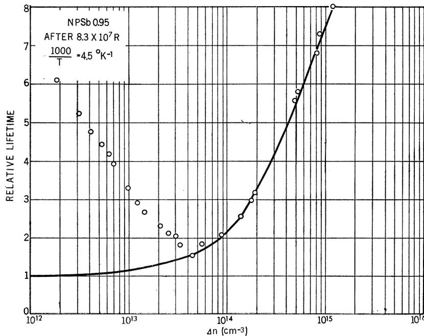
FIG. 5. The dependence of lifetime on excess density at  $-51^\circ\text{C}$ , for 0.95- $\Omega$  cm Sb-doped Ge following  $\gamma$  irradiation.
