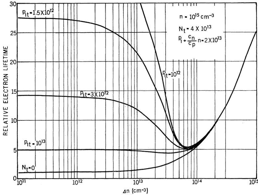
FIG. 1. Examples of the dependence of electron lifetime on excess electron density. It is assumed that the recombination and trapping centers lie below the Fermi level, and  $c_p \gg c_n$ .
