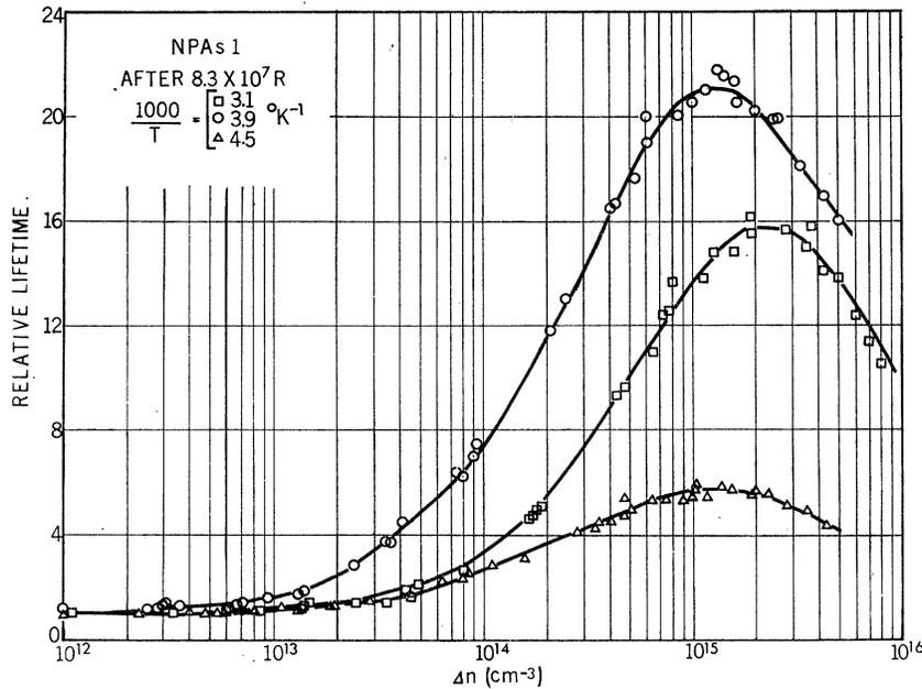
FIG. 4. The dependence of lifetime on excess density at three different temperatures for 1- $\Omega$  cm As-doped Ge following  $\gamma$  irradiation.
