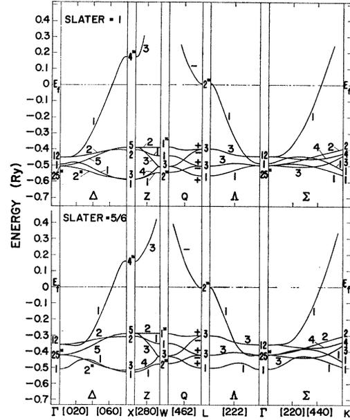
FIG. 1.  $E(\mathbf{k})$  curves for self-consistent silver in directions of high symmetry, for "Slater = 1" and "Slater =  $\frac{5}{6}$ ," shifted so that  $E_f = 0.0$  Ry.
