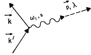
FIG. 3. Feynman diagram for the resonant process involving surface plasmon excitation followed by radiative decay.
