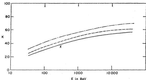
FIG. 5. Nucleon inelasticities derived from the model of nucleon-nucleon interactions. The dashed line represents the results when the mesons are emitted isotropically; the solid line gives the results for a distribution of the form  $1-0.5 \cos\theta$ . The upper curve represents an estimate of the inelasticity for nucleon-nucleus interactions with nitrogen or oxygen. The cross shows the experimental result of Dobrotin *et al.* (see Ref. 7).
