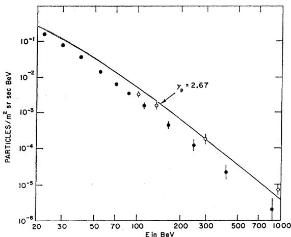
FIG. 8. The muon flux from the zenith as measured at sea level. The solid points represent the results of the Durham group (see Ref. 12) and the open points are from the Manchester results (see Ref. 13). The solid curve shows the flux as calculated on the basis of this model.
