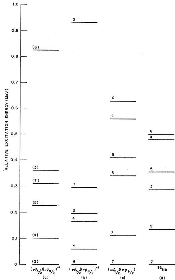
FIG. 9. (a) Particle-hole spectrum deduced from this work for the  $(\nu d_{5/2})(\nu g_{9/2})^{-1}$  interaction. These assignments must be considered very tentative. (b) Particle-hole spectrum for the  $(\nu d_{5/2})(\pi g_{9/2})^{-1}$  interaction as calculated from the particle-particle interaction shown in (c). (c)  $(\nu d_{5/2})(\pi g_{9/2})$  particle-particle interaction deduced from the observed spectrum of  $^{92}\text{Nb}$  shown in (d).
