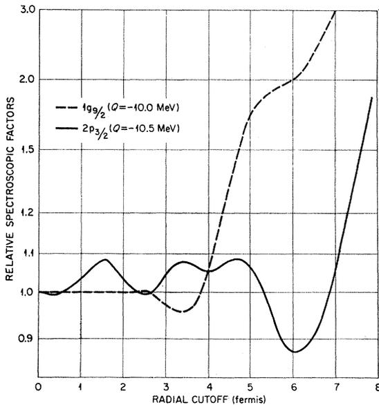
FIG. 3. Relative spectroscopic factors for  $1g_{9/2}$  and  $2p_{3/2}$  neutron pickup as a function of cutoff of the radial integral. Each curve has been normalized to unity at zero cutoff.
