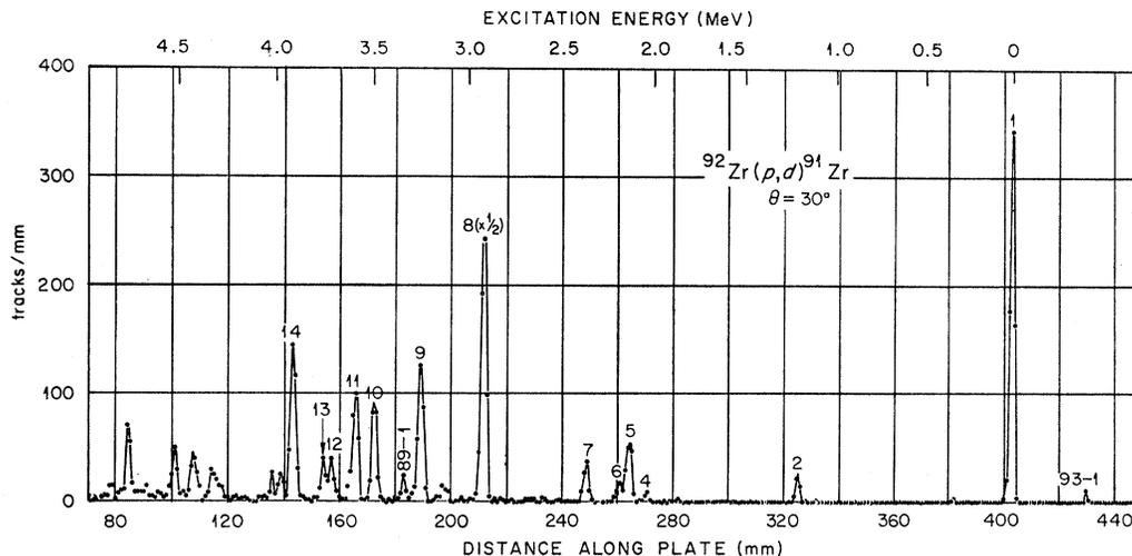
FIG. 8. Spectrum for  $^{92}\text{Zr}(p,d)^{91}\text{Zr}$  at  $30^\circ$ . The ground state corresponds to a  $Q$  value of  $-6.44 \pm 0.04$  MeV.
