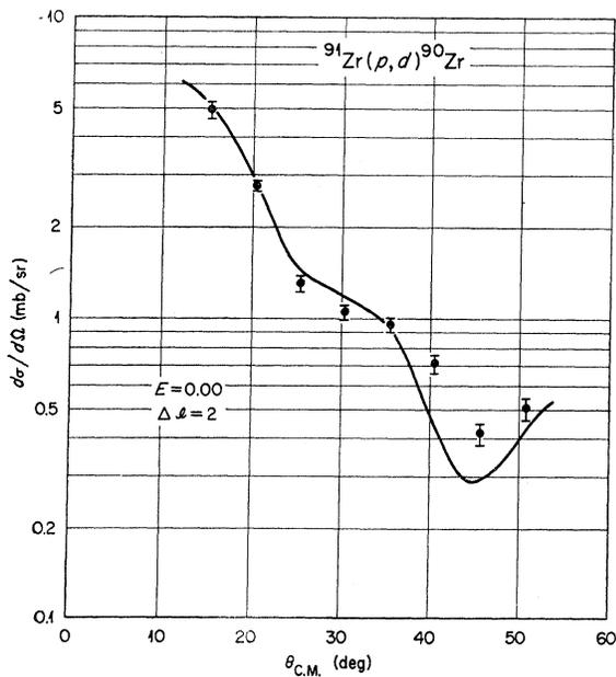
FIG. 7. Angular distribution of the deuteron group leading to the ground state in the reaction  $^{91}\text{Zr}(p,d)^{90}\text{Zr}$ . The solid curve is the DWBA calculation.
