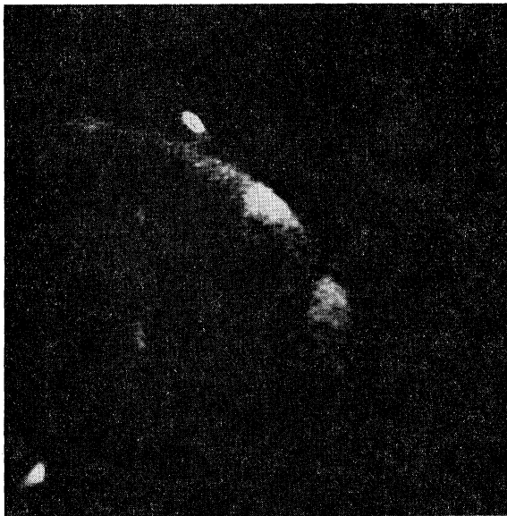
FIG. 3. A two-dimensional energy spectrum of E_{Be^8}(E_A + E_B) versus E_\alpha(E_C) for the C^{13}(He^3, 4\alpha) reactions at \theta_{AB} = +48^\circ and \theta_C = -105^\circ and E_{He^3} = 5.00 MeV.
