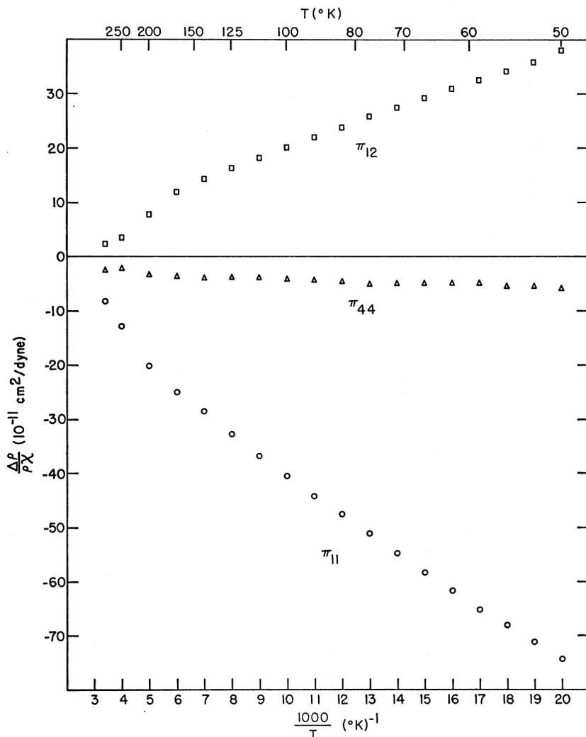
FIG. 5. Average values of the piezoresistance tensor components at integral values of  $1000/T$ . These were obtained by drawing a best-fit curve through the measured  $\Delta\rho/\rho\chi$  values. The intersections of the best-fit curves with integral values of  $1000/T$  were averaged for each component. The component  $\pi_{44}$  was determined by combining the quantities  $\pi_{11}$ ,  $\pi_{12}$ , and  $\frac{1}{2}(\pi_{11} + \pi_{12} + \pi_{44})$ .
