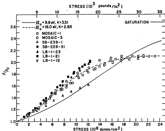
FIG. 10. High-stress piezoresistance measurements on  $Mg_2Sn$  at 77°K. The solid line indicates the expected result based on Eq. (5) with  $\epsilon_u = 9.8$  eV and  $K = 3.51$ . The dashed curve shows the best fit to experimental data with  $\epsilon_u = 18$  eV and  $K = 2.65$ .
