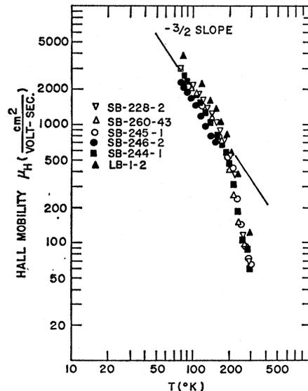
FIG. 3. Hall mobility of some piezoresistance samples of Mg<sub>2</sub>Sn. The  $-\frac{3}{2}$  slope indicates that acoustic mode scattering dominates in the extrinsic temperature region.
