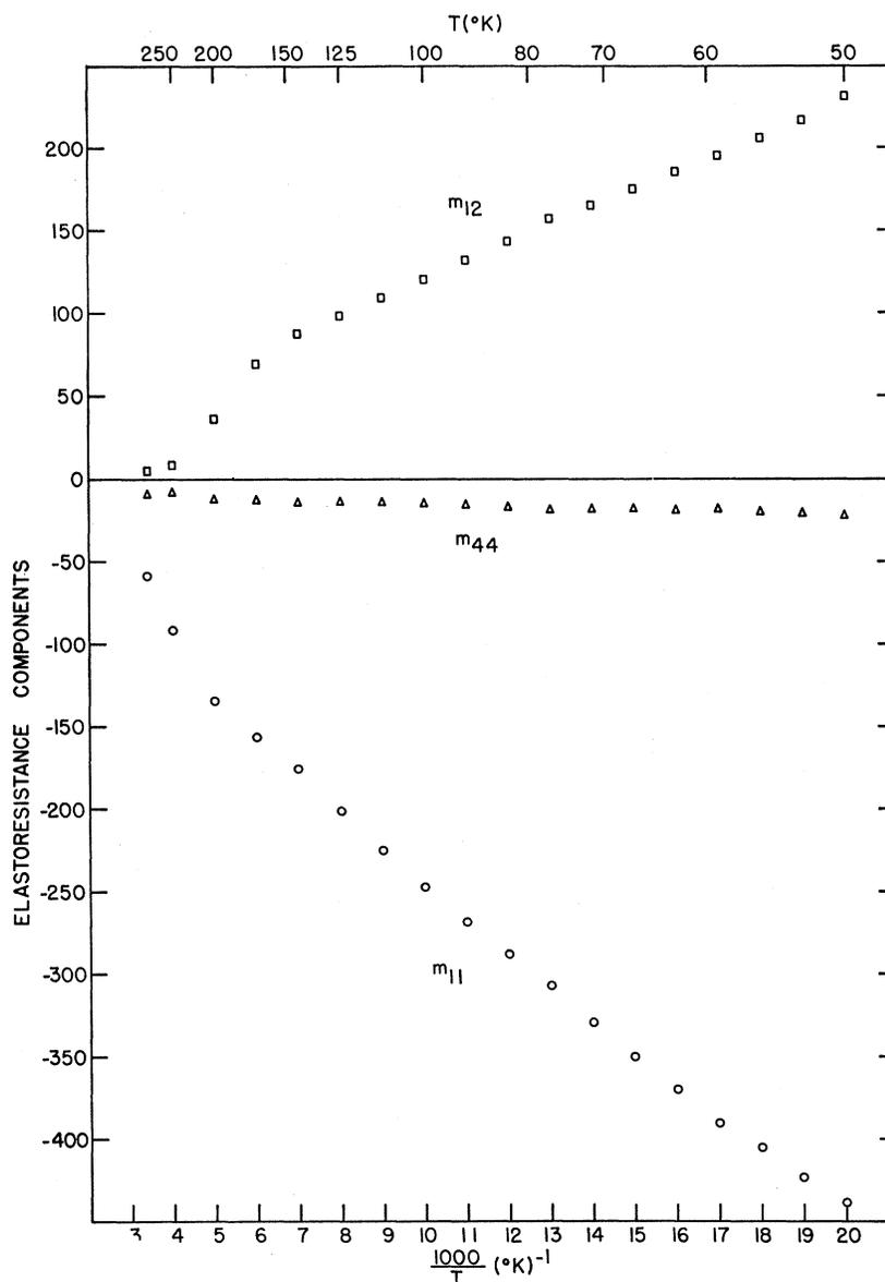
FIG. 7. Elasto-resistance tensor components for  $Mg_2Sn$  determined from the piezoresistance components in Fig. 5 and the elastic constants of Davis *et al.* (Ref. 5).
