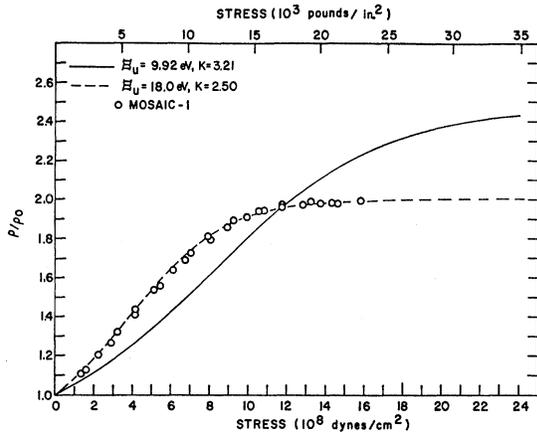
FIG. 11. High-stress piezoresistance measurements on sample mosaic-1 at 50°K. The solid line indicates the expected result based on Eq. (5) with  $\epsilon_u = 9.9$  eV and  $K = 3.21$ . The dashed curve shows the best fit to experimental data with  $\epsilon_u = 18$  eV and  $K = 2.50$ .
