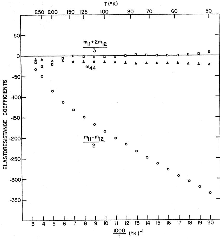
FIG. 8. Elasto-resistance coefficients of Mg<sub>2</sub>Sn. The volume coefficient,  $\frac{1}{3}(m_{11}+2m_{12})$ , and one of the shear coefficients  $m_{44}$  are small and temperature-independent in the extrinsic temperature region. The other shear coefficient  $\frac{1}{2}(m_{11}-m_{12})$  is large and decreases with decreasing temperature. These results suggest energy ellipsoids in the (100) directions.
