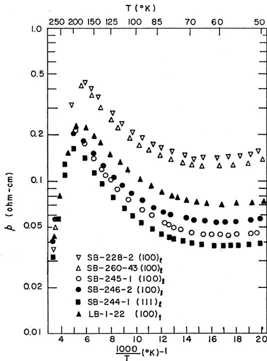
FIG. 1. Electrical resistivity of some piezoresistance samples of Mg<sub>2</sub>Sn.
