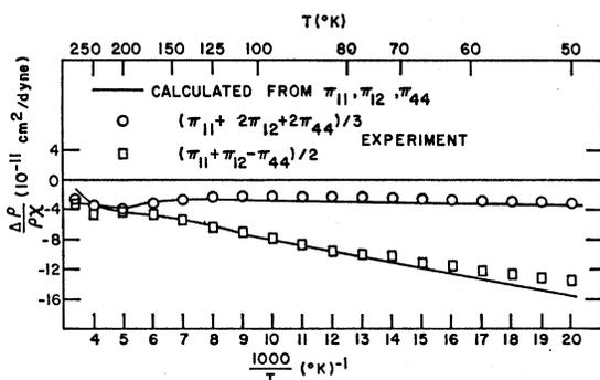
FIG. 6. Comparison of the observed components  $\frac{1}{3}(\pi_{11} + 2\pi_{12} + 2\pi_{44})$  and  $\frac{1}{2}(\pi_{11} + \pi_{12} - \pi_{44})$  with the values calculated with  $\pi_{11}$ ,  $\pi_{12}$ , and  $\pi_{44}$  obtained from Fig. 5. The good agreement indicated that the piezoresistance results were internally consistent.
