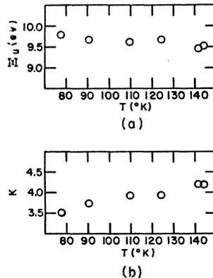
FIG. 9. Temperature dependence of the deformation potential (a) as determined with the use of the mobility anisotropy (b) found by Umeda (Ref. 1).
