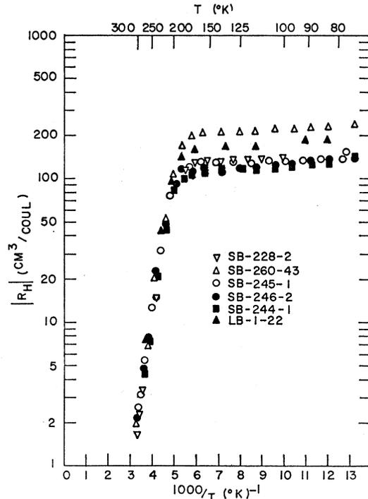
FIG. 2. Hall coefficient of some piezoresistance samples of Mg<sub>2</sub>Sn.
